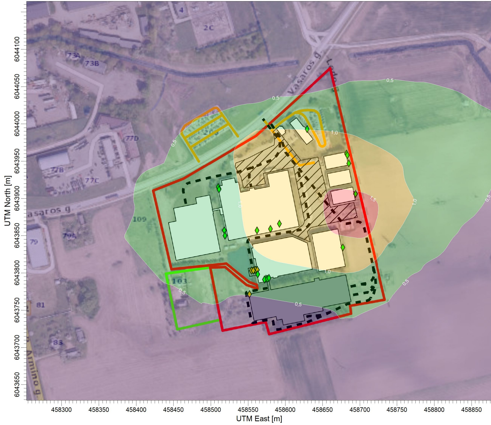
PLOT FILE OF ANNUAL VALUES AVERAGED ACROSS 5 YEARS FOR SOURCE GROUP: PUV Max: 1,8 [ug/m 3 ] at (458708,75, 6043870,53)
