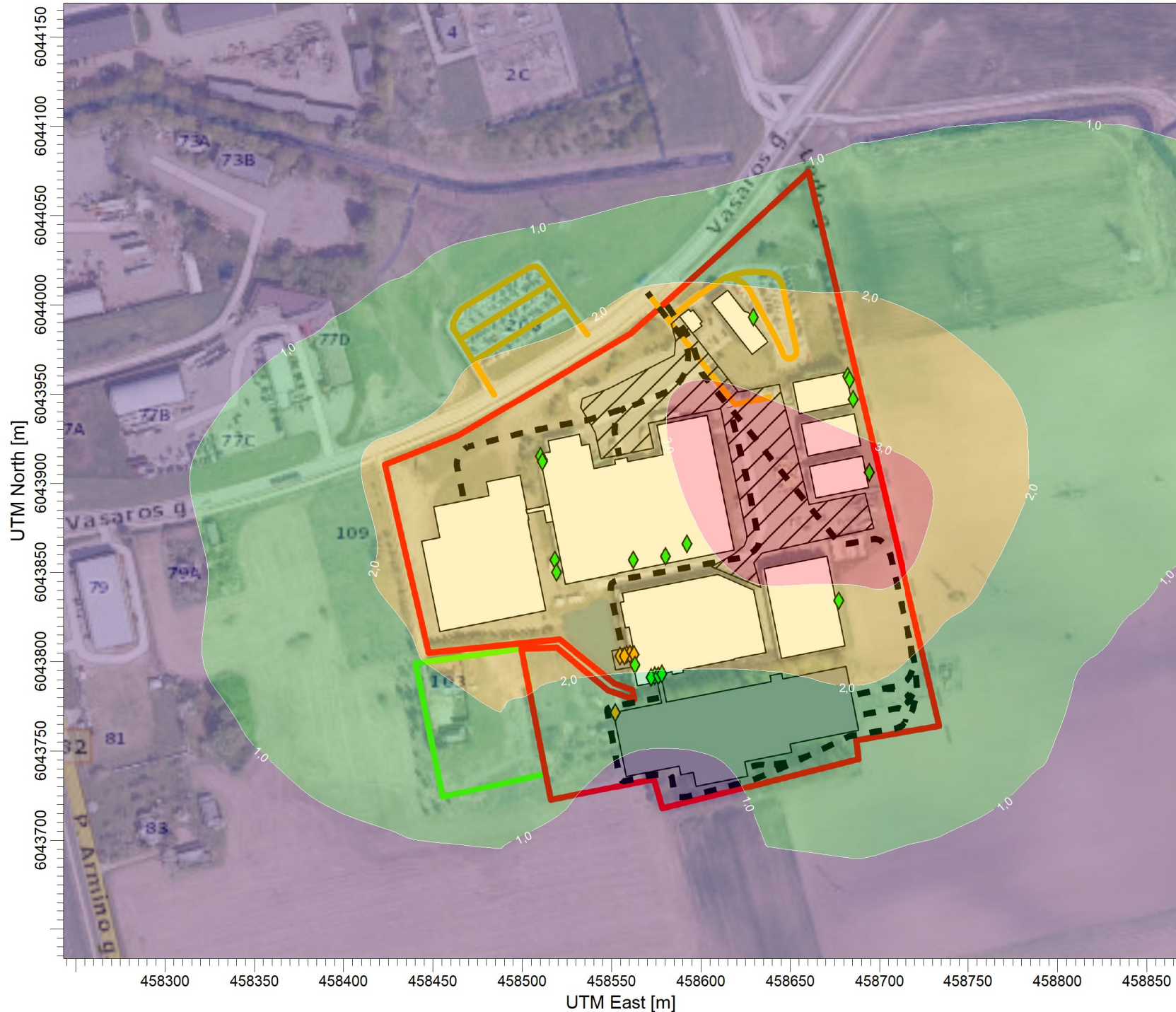
PLOT FILE OF 90.40TH PERCENTILE 24-HR VALUES FOR SOURCE GROUP: PUV Max: 3,6 [ug/m^3] at (458708,75, 6043870,53)
