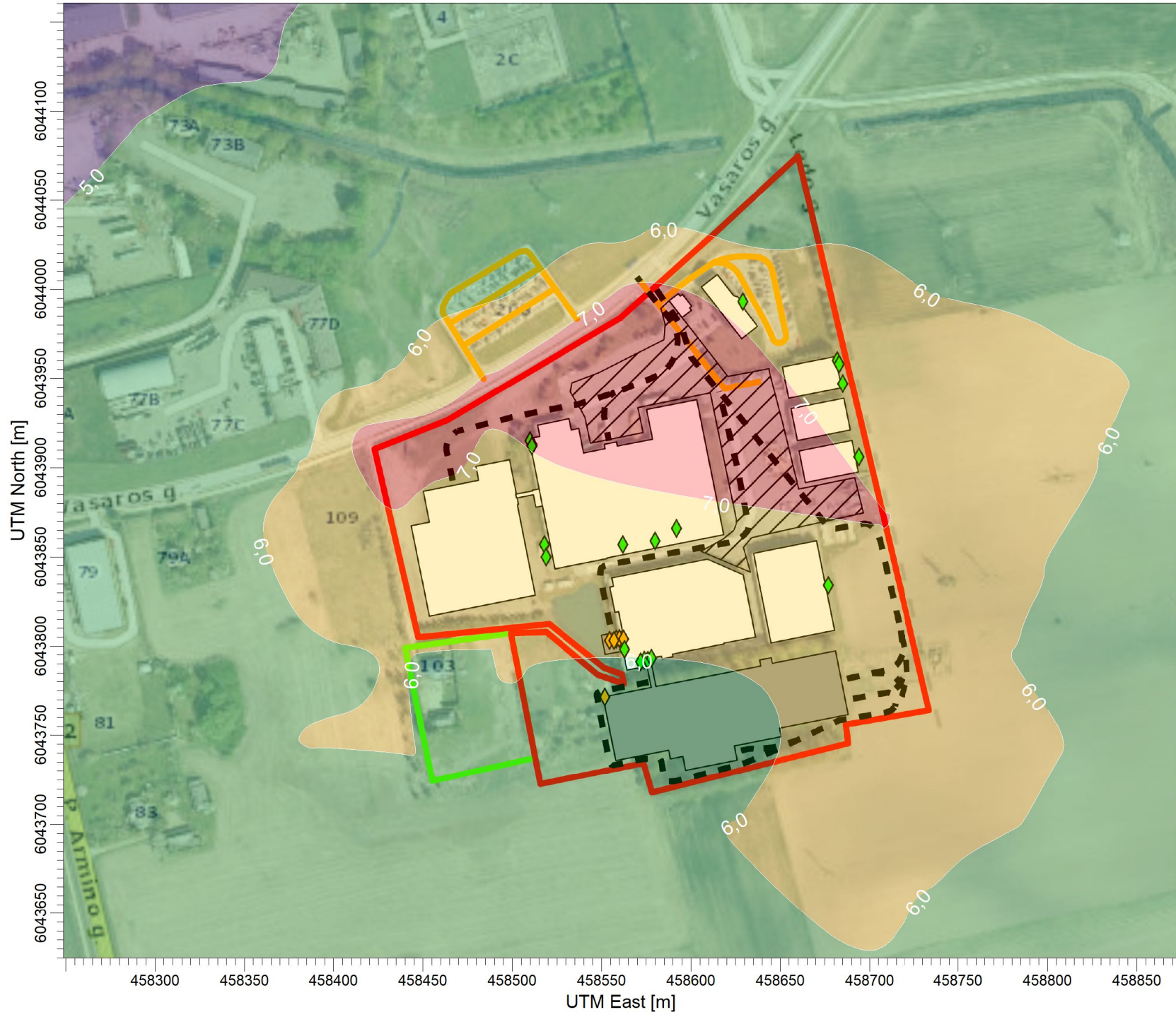
PLOT FILE OF 99.70TH PERCENTILE 1-HR VALUES FOR SOURCE GROUP: ALL Max: 7,8 [ug/m^3] at (458559,61, 6043982,26)
