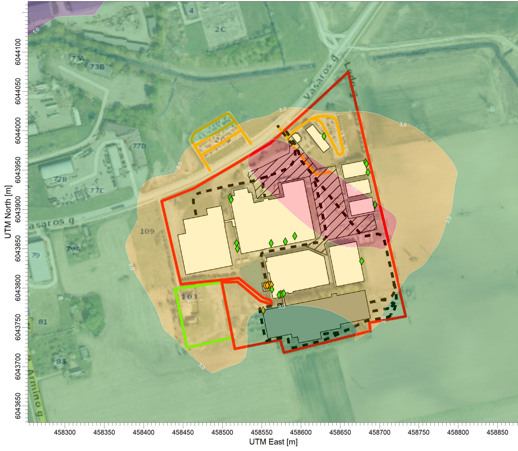
PLOT FILE OF 99.20TH PERCENTILE 24-HR VALUES FOR SOURCE GROUP: PUV Max: 5,5 [ug/m^3] at (458708,75, 6043870,53)
