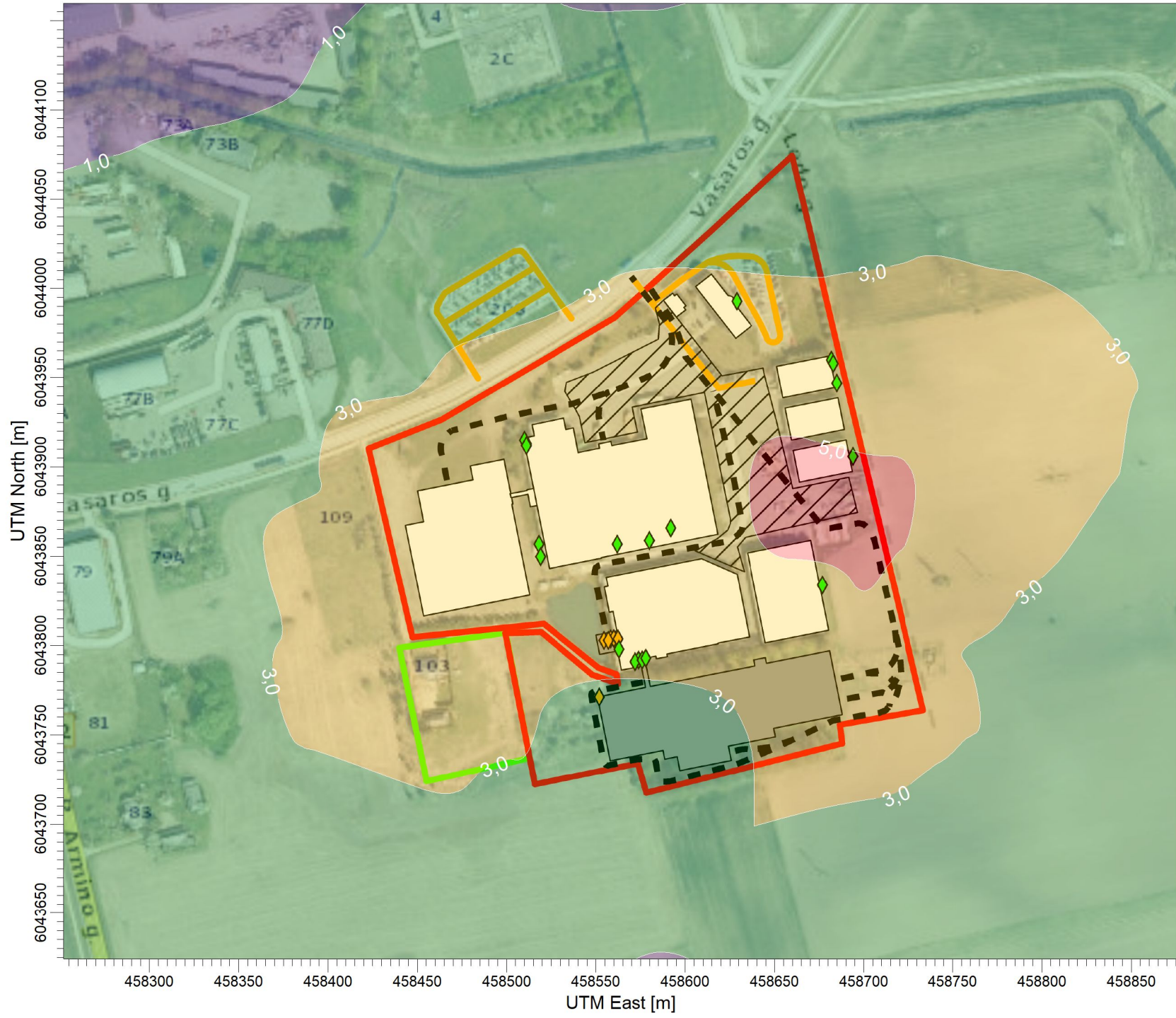
PLOT FILE OF 98.50TH PERCENTILE 1-HR VALUES FOR SOURCE GROUP: ALL Max: 5,7 [ug/m^3] at (458708,75, 6043870,53)
