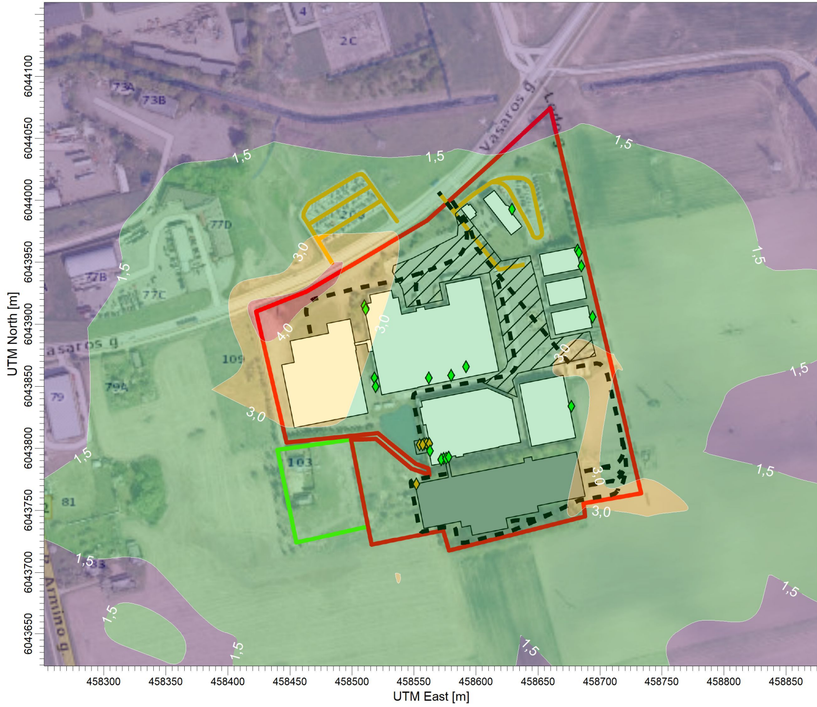
PLOT FILE OF HIGH 1ST HIGH 24-HR VALUES FOR SOURCE GROUP: ALL Max: 4,5 [ \mu\text{g}/\text{m}^3 ] at (458423,64, 6043911,11)
