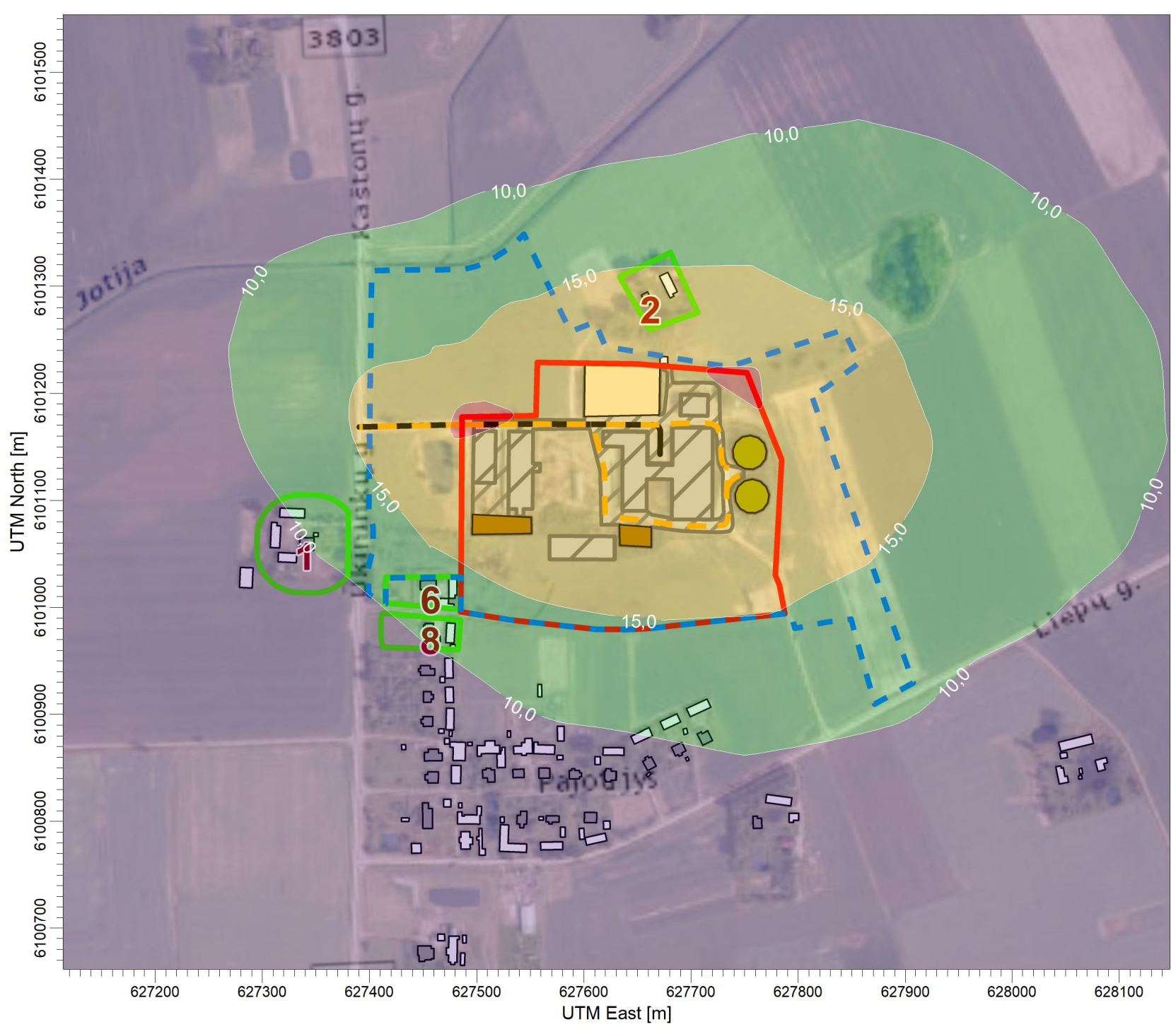
PLOT FILE OF 99.80TH PERCENTILE 1-HR VALUES FOR SOURCE GROUP: ALL Max: 27,3 [ \mu\text{g}/\text{m}^3 ] at (627486,97, 6101177,43)
