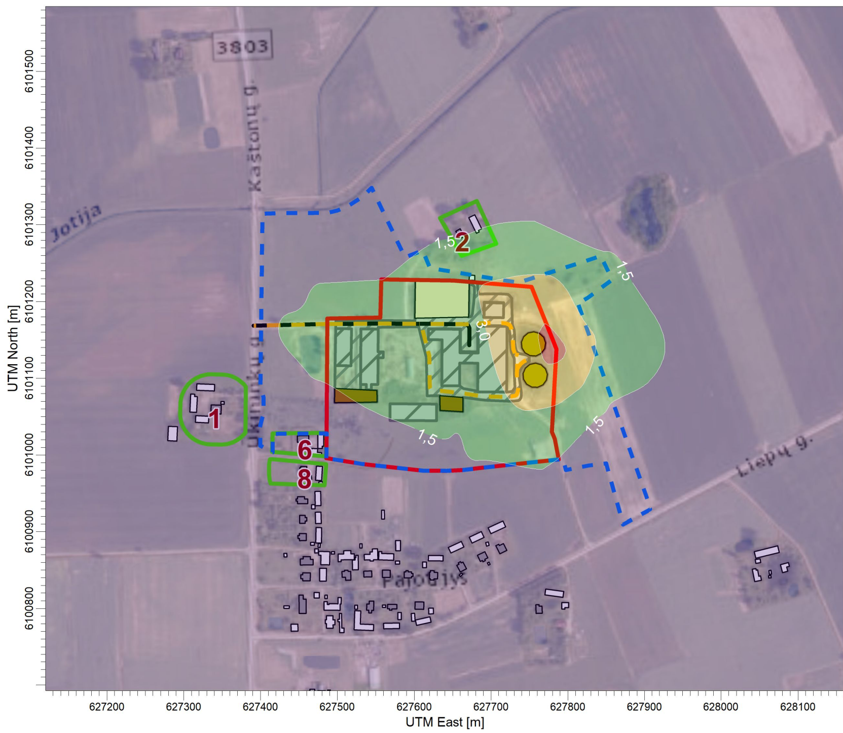
PLOT FILE OF 99.20TH PERCENTILE 24-HR VALUES FOR SOURCE GROUP: PUV Max: 5,0 [ug/m^3] at (627785,47, 6101138,61)
