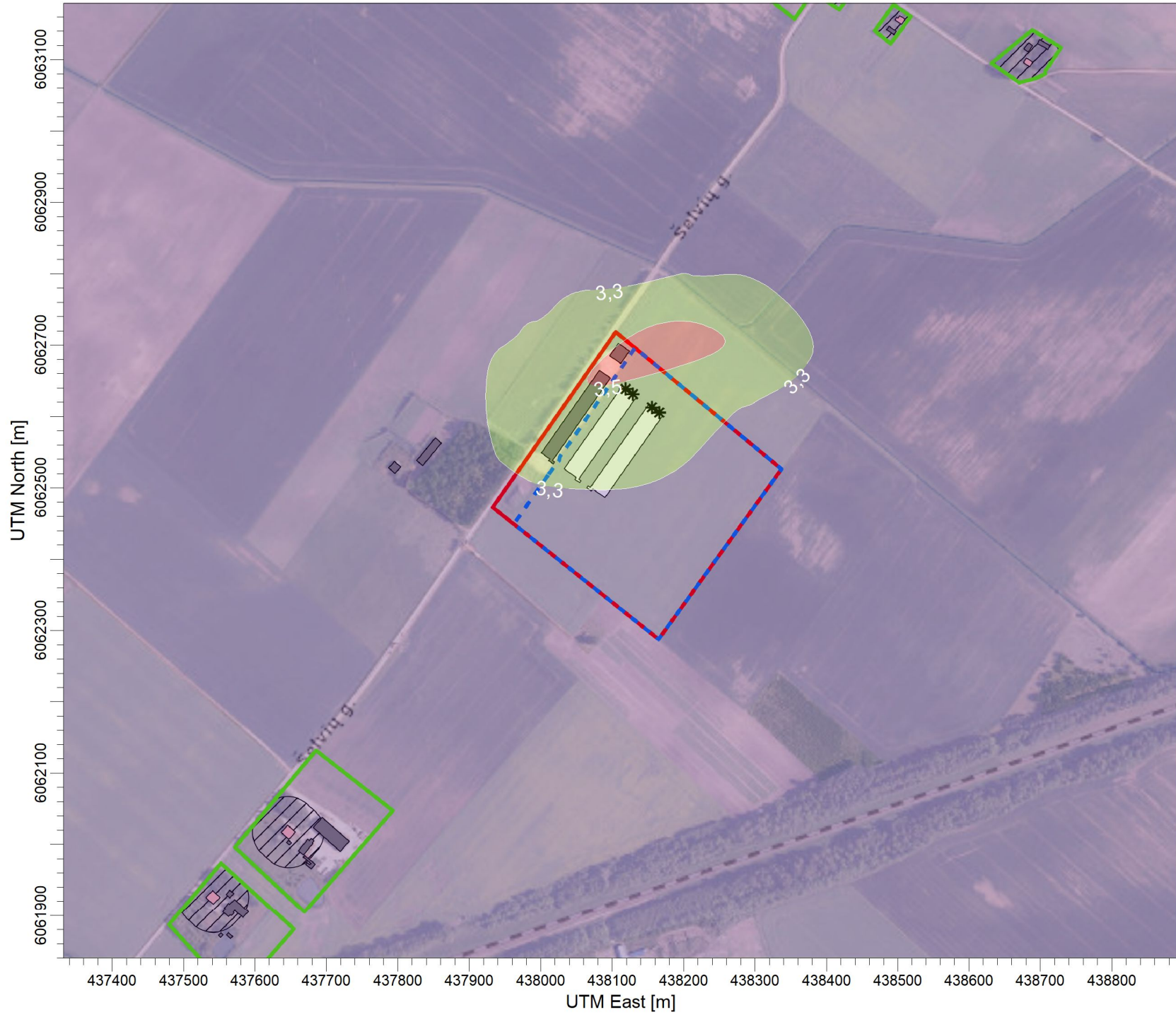
PLOT FILE OF ANNUAL VALUES AVERAGED ACROSS 5 YEARS FOR SOURCE GROUP: ALL Max: 3,6 [ug/m^3] at (438201,95, 6062709,88)
