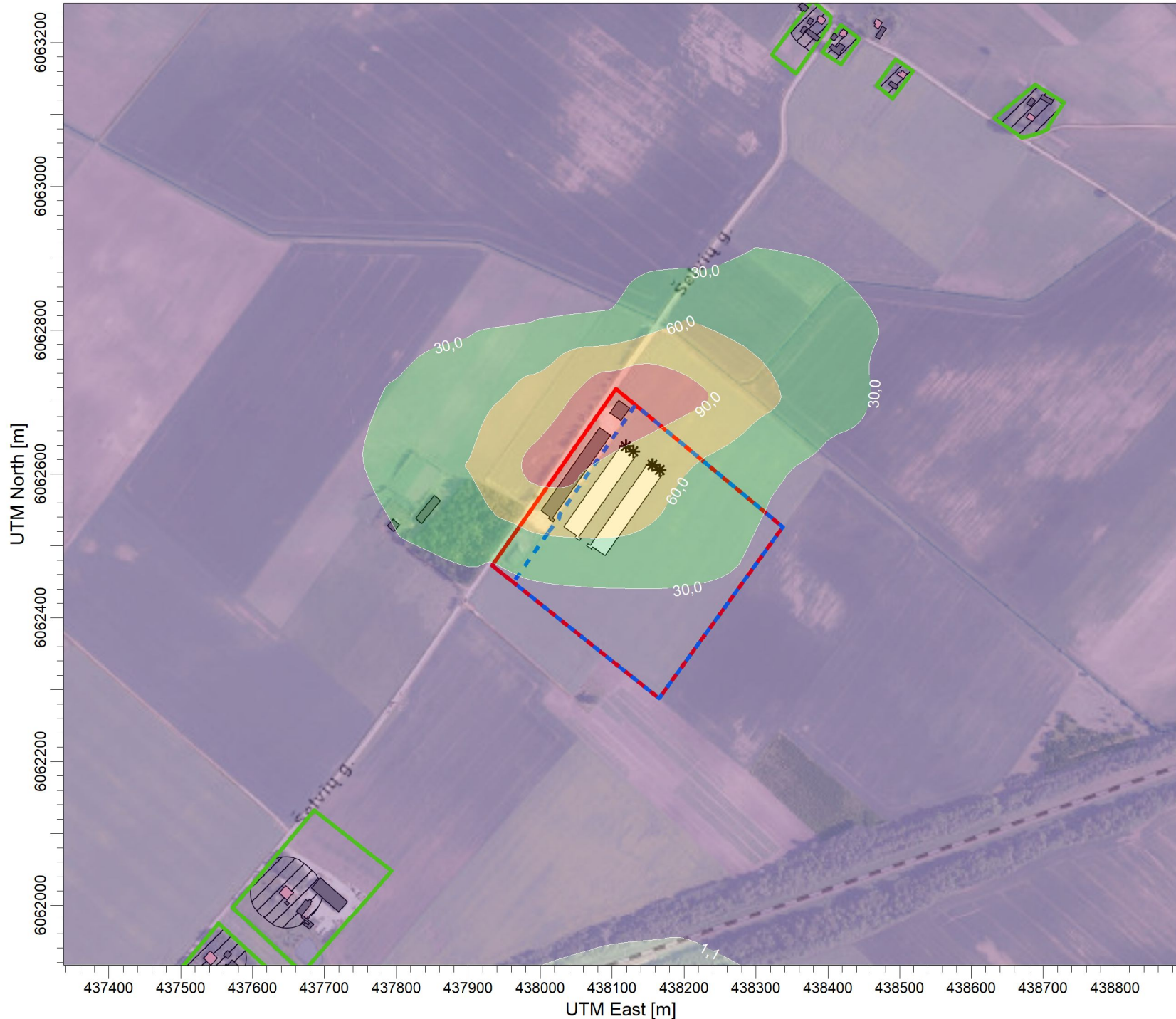
PLOT FILE OF 98.50TH PERCENTILE 1-HR VALUES FOR SOURCE GROUP: ALL Max: 111,5 [ug/m 3 ] at (438105,70, 6062717,46)
