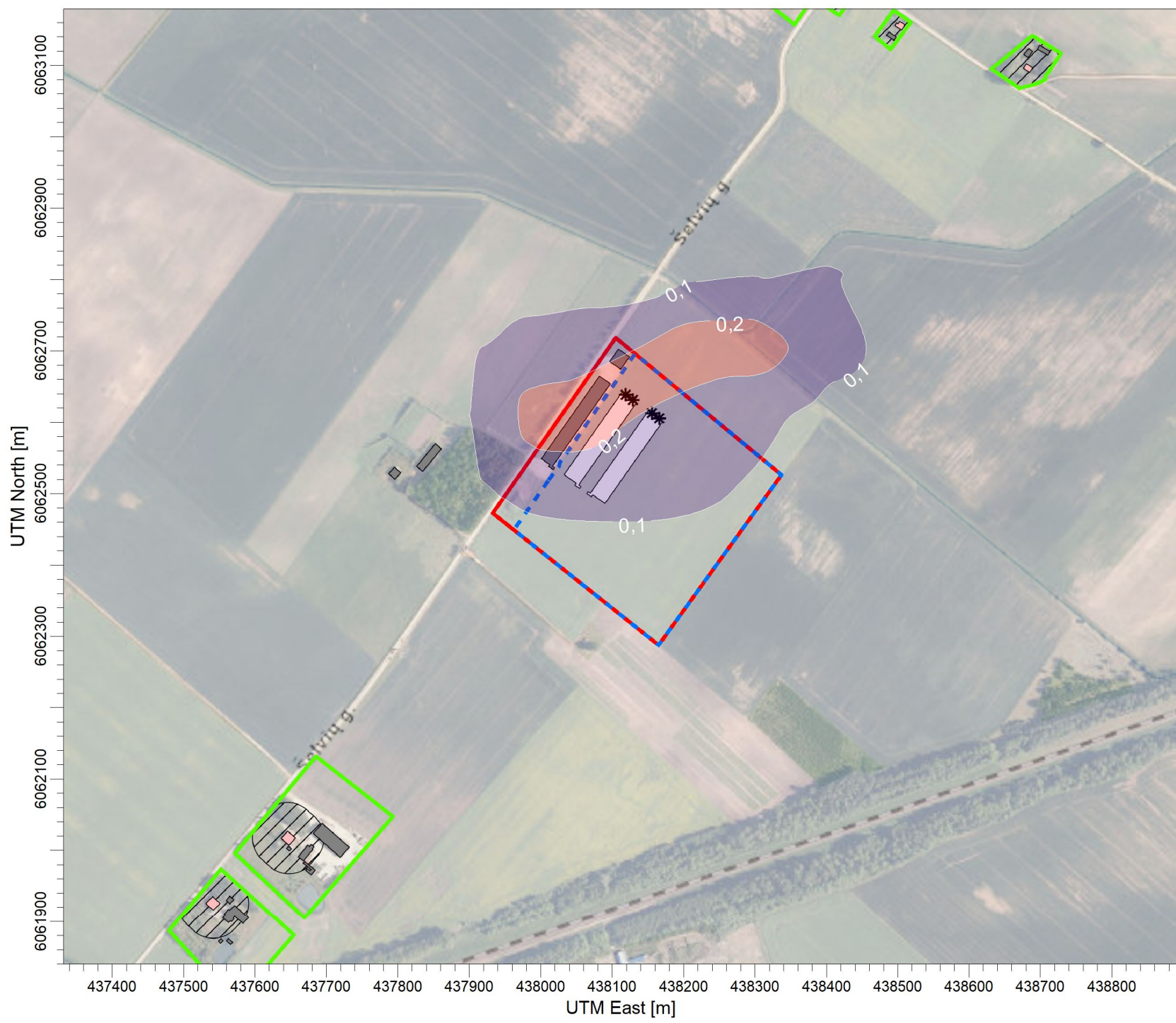
PLOT FILE OF ANNUAL VALUES AVERAGED ACROSS 5 YEARS FOR SOURCE GROUP: PŪV Max: 0,3 [ug/m^3] at (438301,95, 6062709,88)
