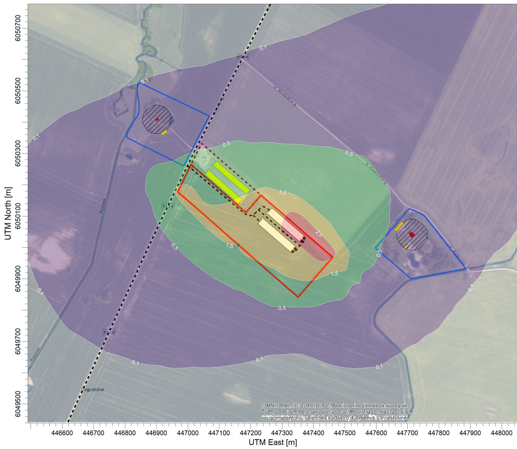
PLOT FILE OF ANNUAL VALUES AVERAGED ACROSS 5 YEARS FOR SOURCE GROUP: PUV Max: 3,0 [ug/m^3] at (447353,30, 6050081,72)
