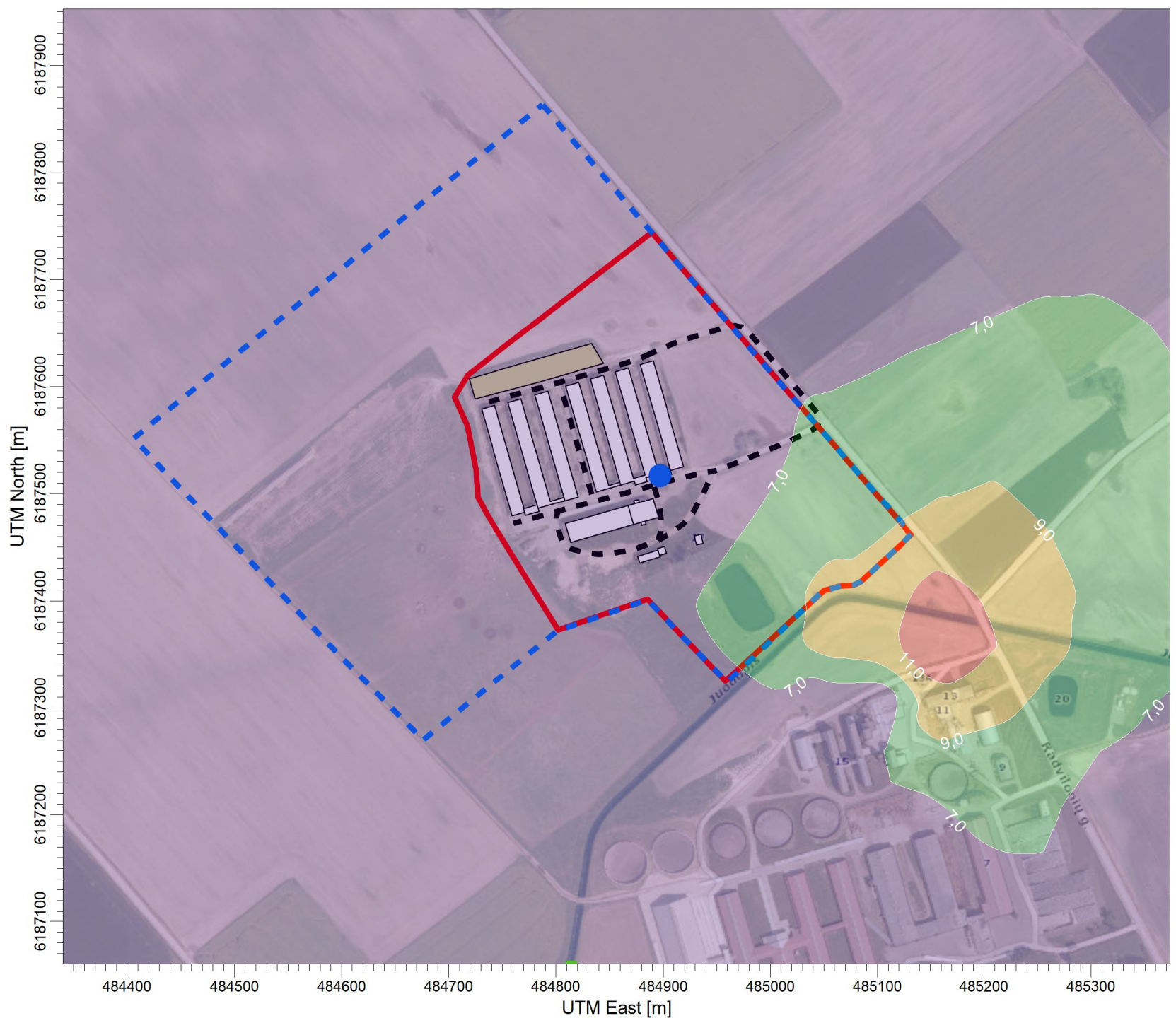
ug/m 3 PLOT FILE OF ANNUAL VALUES AVERAGED ACROSS 5 YEARS FOR SOURCE GROUP: ALL Max: 12,5 [ug/m 3 ] at (485157,88, 6187358,68)
