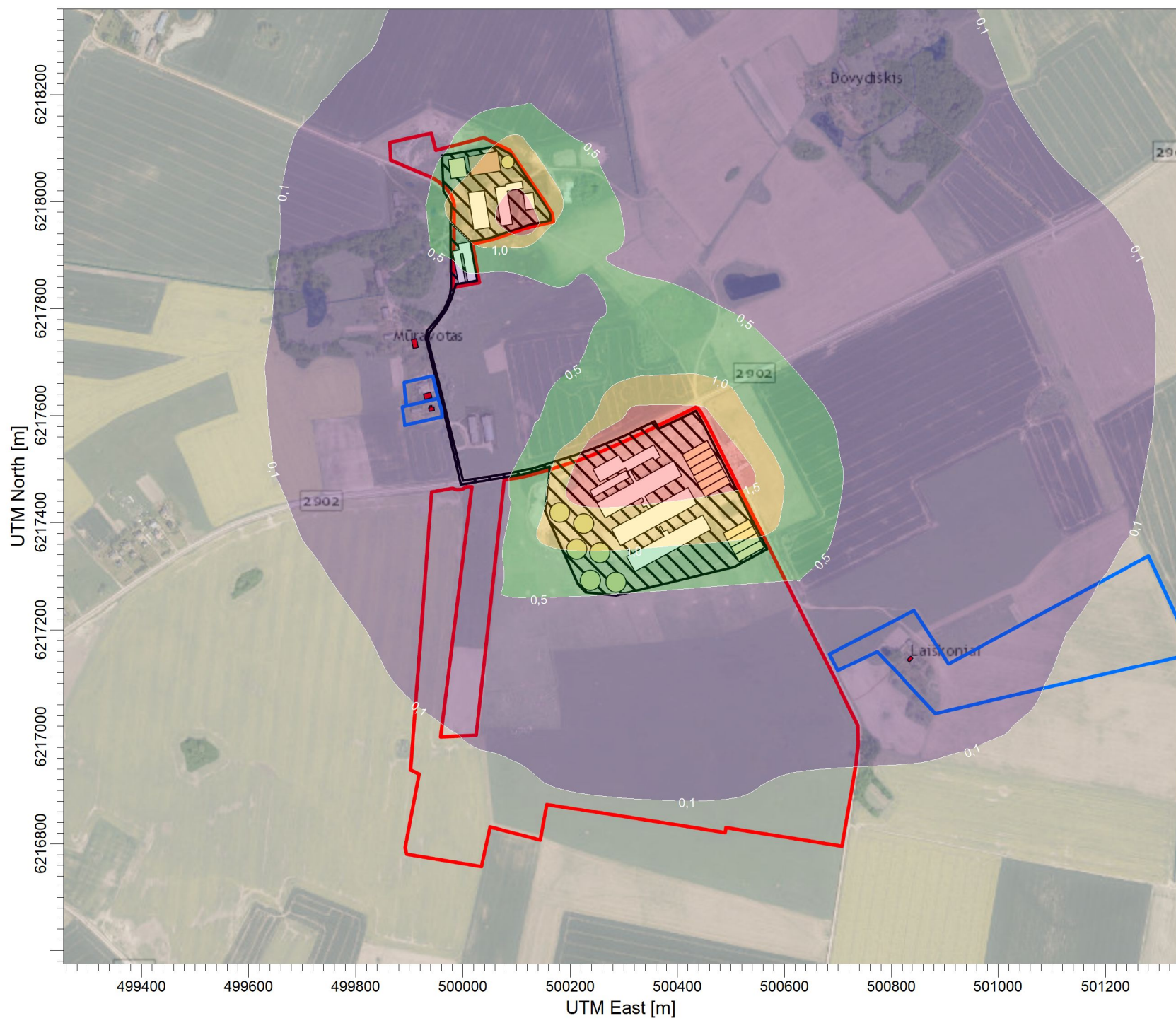
PLOT FILE OF ANNUAL VALUES AVERAGED ACROSS 5 YEARS FOR SOURCE GROUP: PUV Max: 2,1 [ \mu\text{g}/\text{m}^3 ] at (500249,89, 6217530,52)
