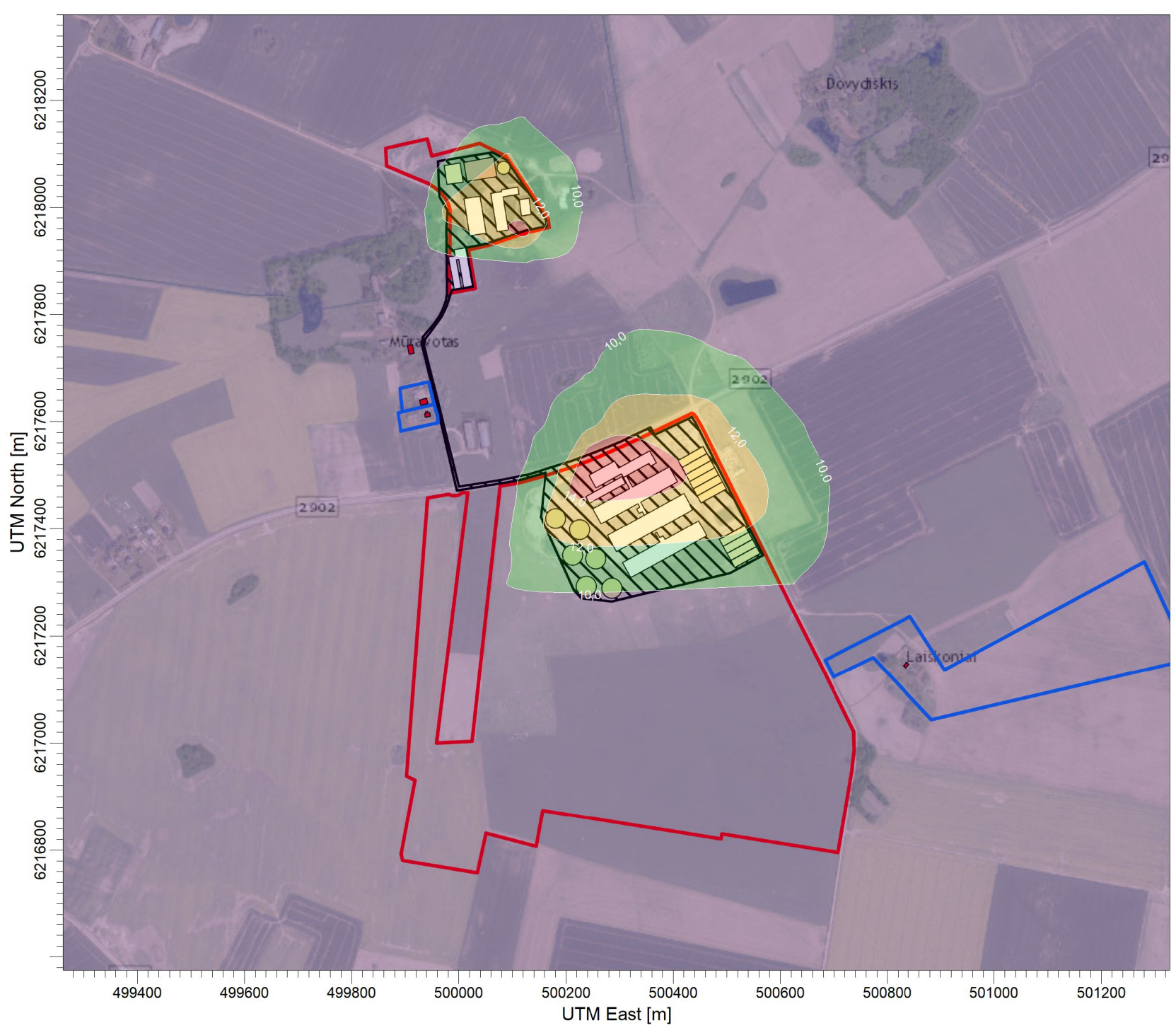
PLOT FILE OF 90.40TH PERCENTILE 24-HR VALUES FOR SOURCE GROUP: ALL Max: 15,9 [ug/m^3] at (500249,89, 6217530,52)
