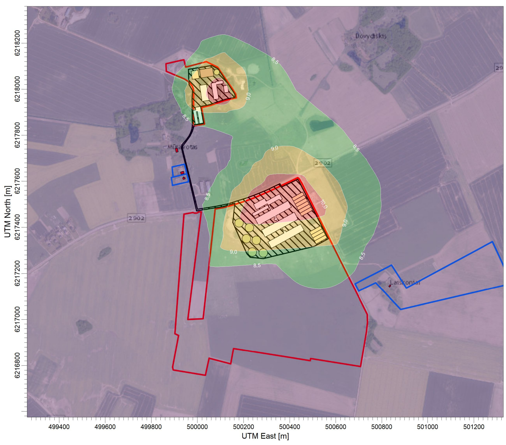
PLOT FILE OF ANNUAL VALUES AVERAGED ACROSS 5 YEARS FOR SOURCE GROUP: ALL Max: 11,0 [ \mu\text{g}/\text{m}^3 ] at (500249,89, 6217530,52)
