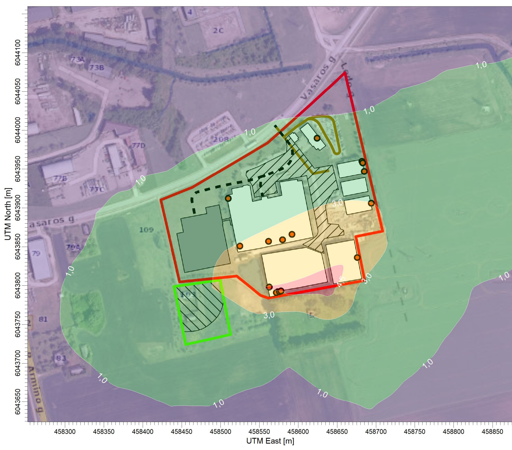
PLOT FILE OF 98.50TH PERCENTILE 1-HR VALUES FOR SOURCE GROUP: ALL Max: 5,1 [ug/m^3] at (458637,13, 6043797,42)
