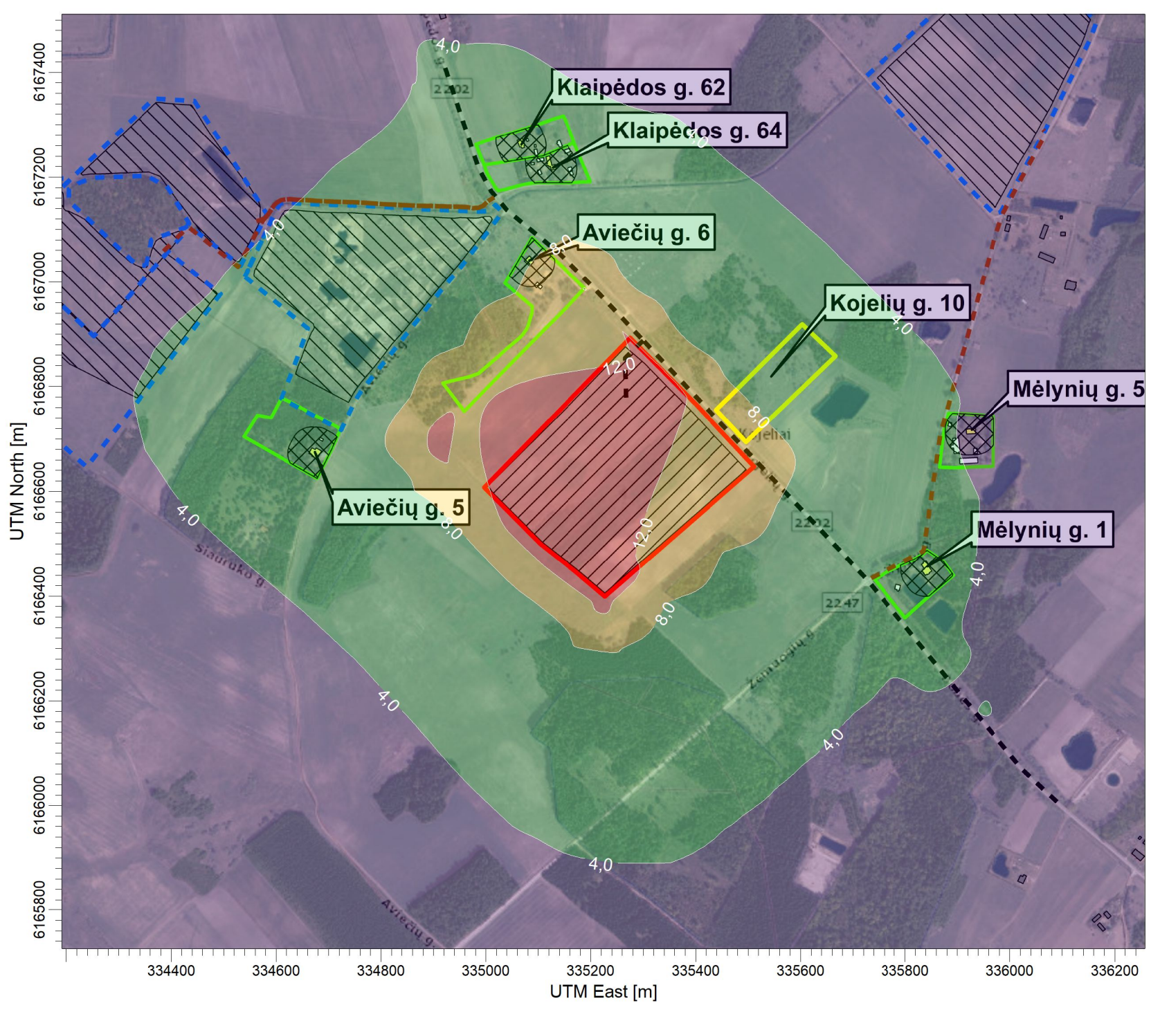
PLOT FILE OF 99.80TH PERCENTILE 1-HR VALUES FOR SOURCE GROUP: PŪV Max: 14,7 [ug/m^3] at (335091,45, 6166508,81)
