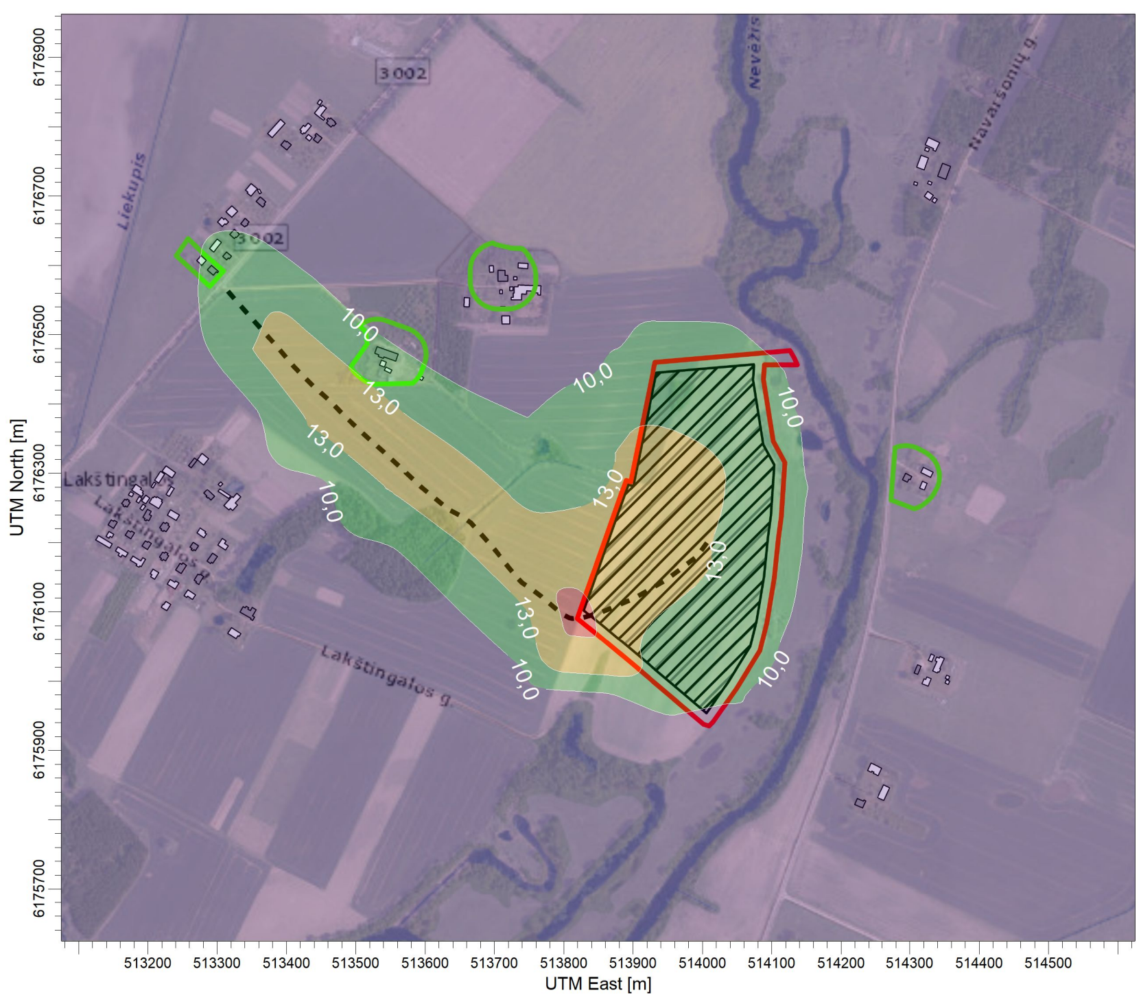
PLOT FILE OF ANNUAL VALUES AVERAGED ACROSS 5 YEARS FOR SOURCE GROUP: ALL Max: 22,0 [ug/m^3] at (513818,95, 6176091,23)
