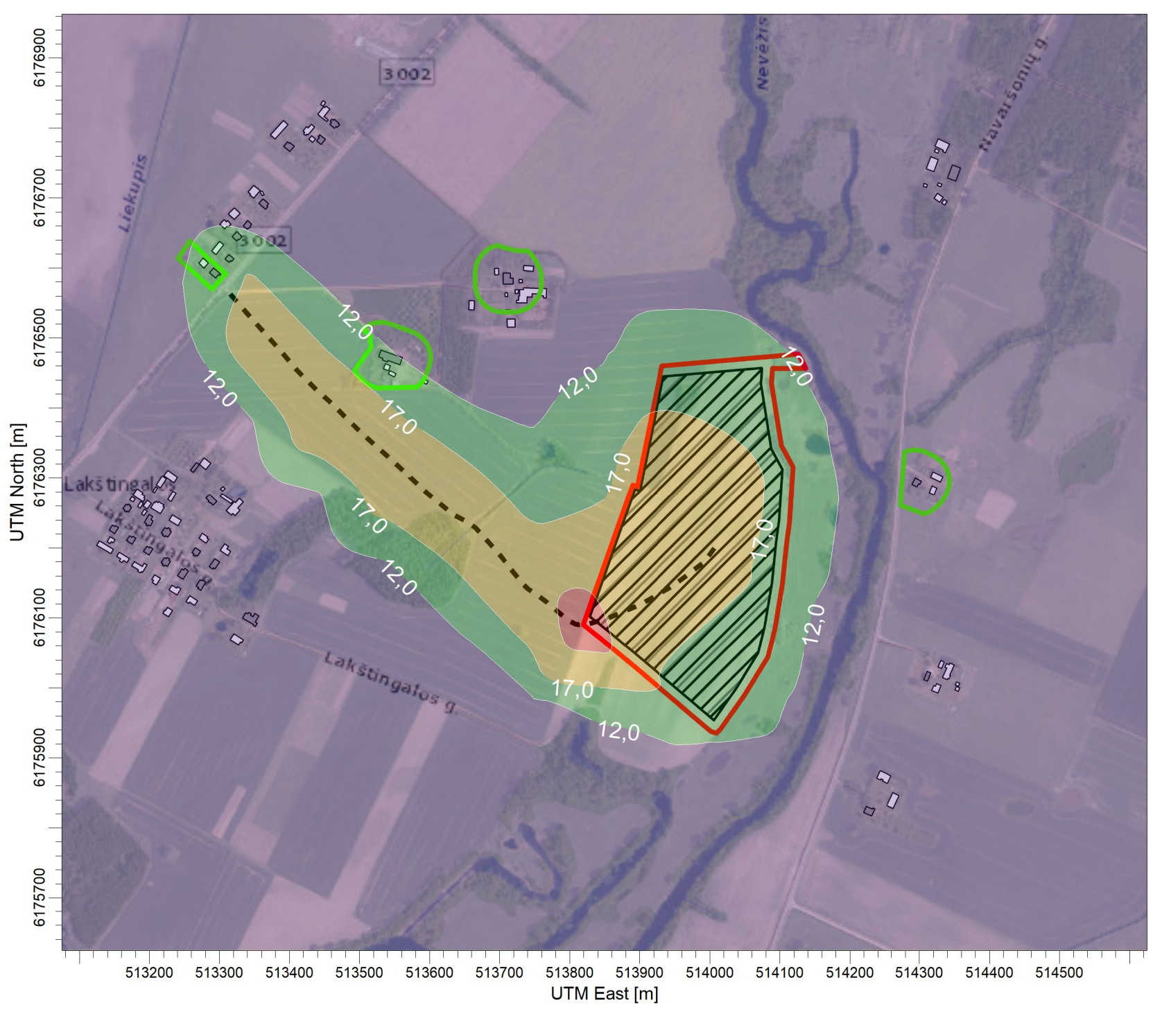
PLOT FILE OF 90.40TH PERCENTILE 24-HR VALUES FOR SOURCE GROUP: ALL Max: 34,6 [ug/m^3] at (513818,95, 6176091,23)
