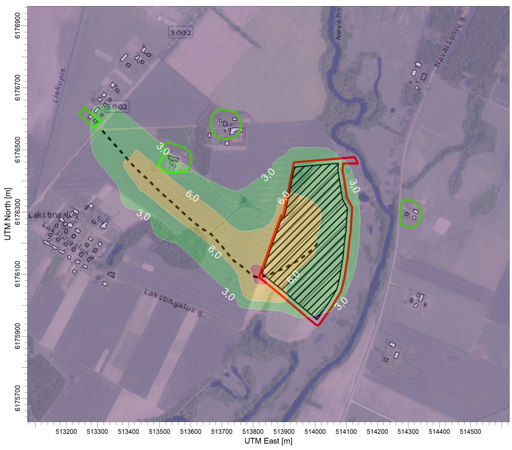
PLOT FILE OF ANNUAL VALUES AVERAGED ACROSS 5 YEARS FOR SOURCE GROUP: PUV Max: 14,8 [ \mu\text{g}/\text{m}^3 ] at (513818,95, 6176091,23)
