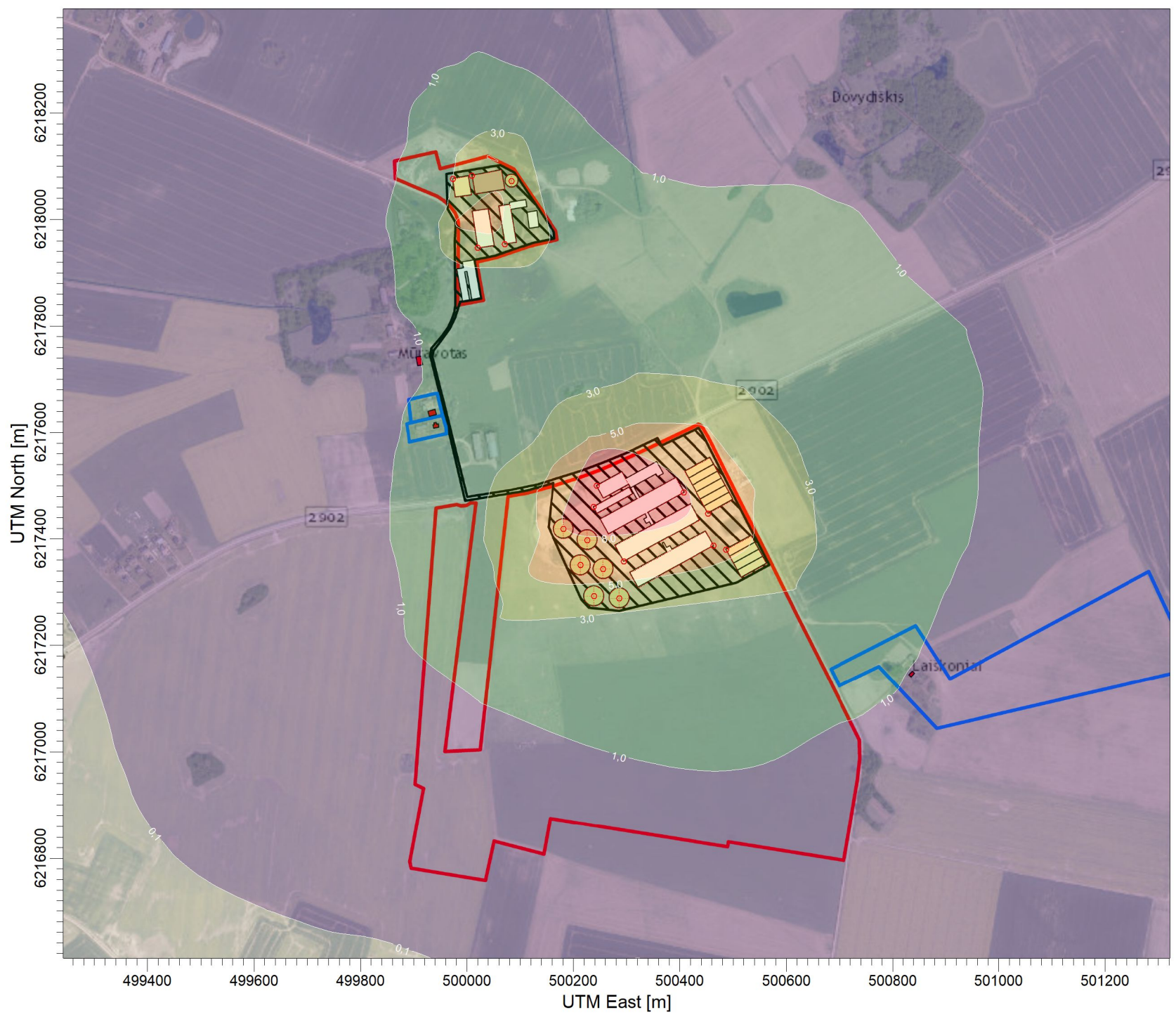
PLOT FILE OF 98.08TH PERCENTILE 1-HR VALUES FOR SOURCE GROUP: ALL Max: 12,4 [OU/M**3] at (500249,89, 6217530,52)
