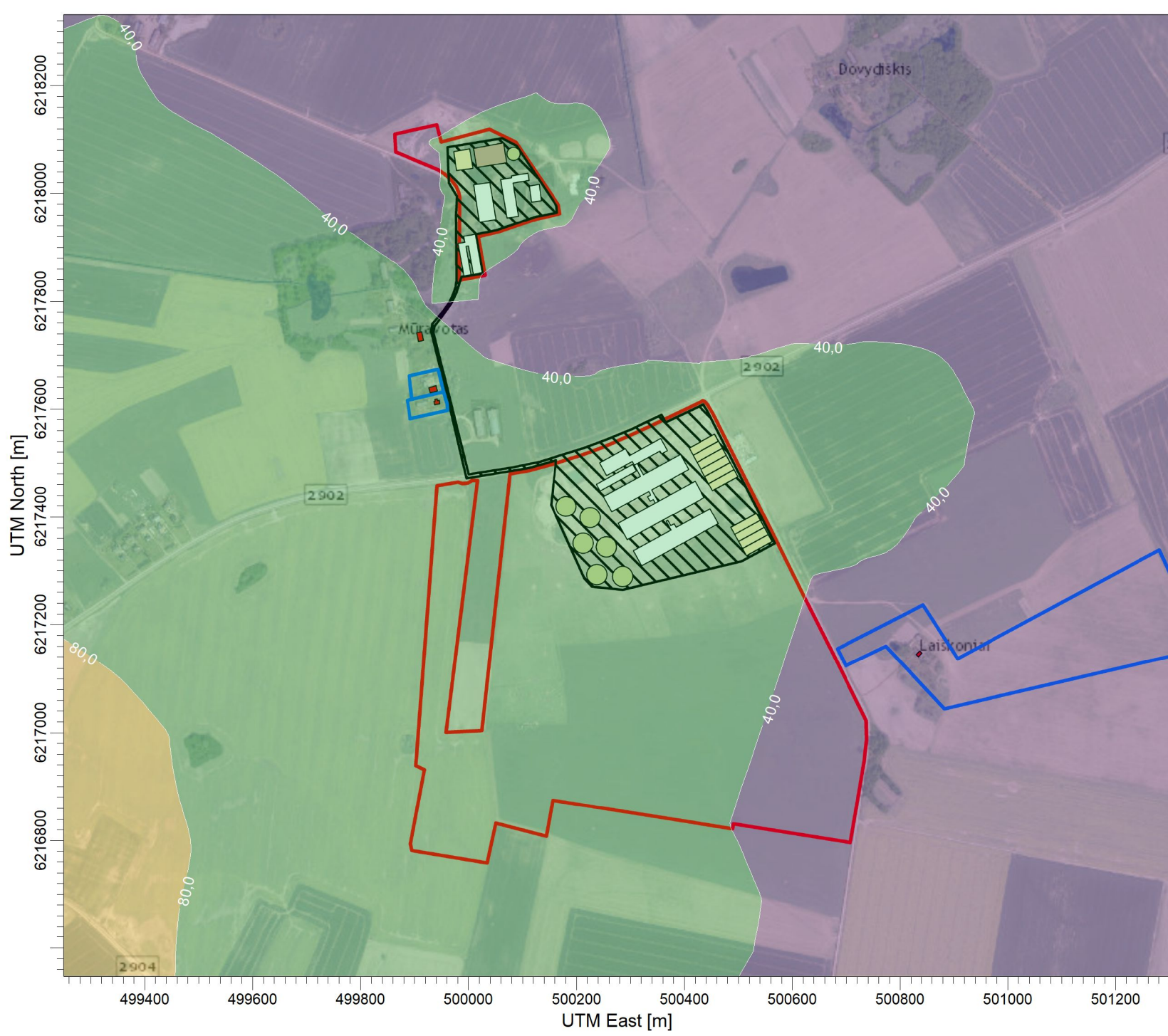
PLOT FILE OF 99.80TH PERCENTILE 1-HR VALUES FOR SOURCE GROUP: ALL Max: 134.2 [ug/m^3] at (498728,00, 6216894,00)
