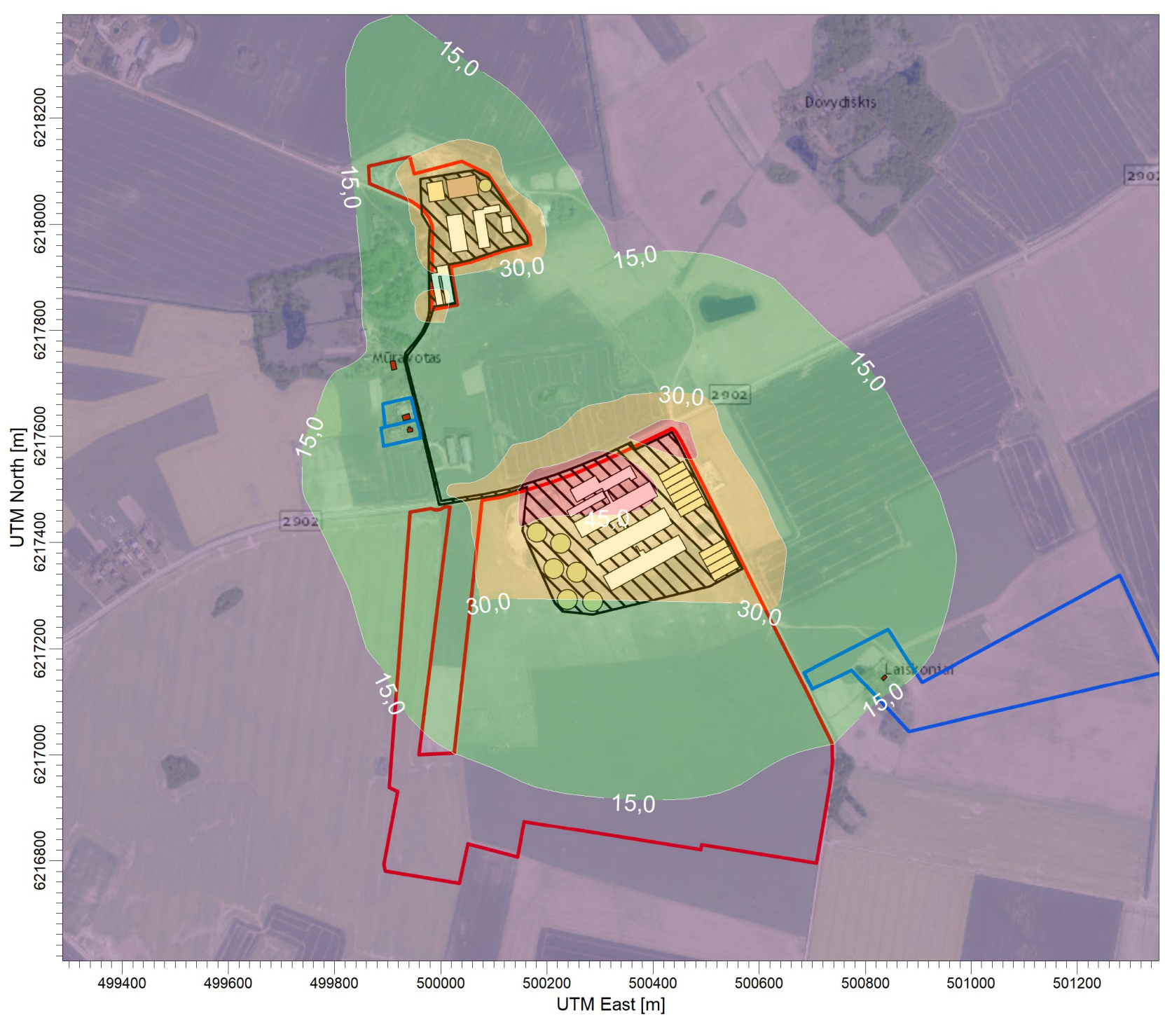
PLOT FILE OF 99.80TH PERCENTILE 1-HR VALUES FOR SOURCE GROUP: PUV Max: 54,0 [ug/m³] at (500193,06, 6217509,58)
