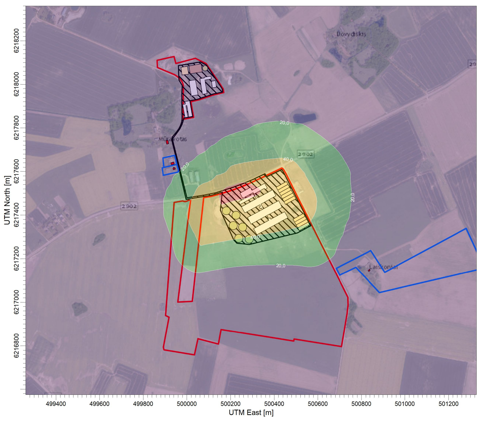
PLOT FILE OF 98.50TH PERCENTILE 1-HR VALUES FOR SOURCE GROUP: ALL Max: 93,7 [ug/m^3] at (500193,06, 6217509,58)
