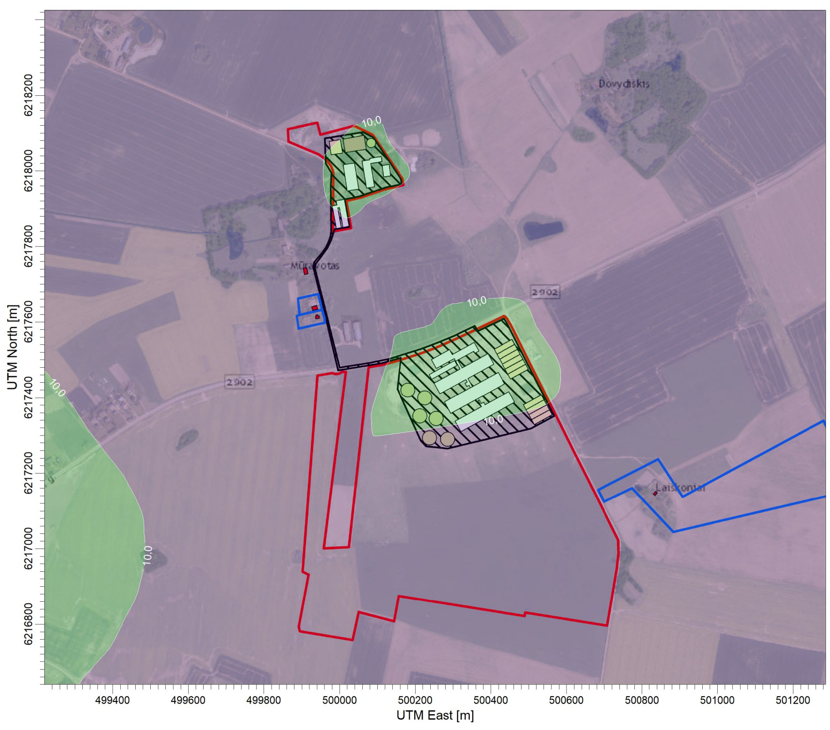
PLOT FILE OF ANNUAL VALUES AVERAGED ACROSS 5 YEARS FOR SOURCE GROUP: ALL Max: 28,9 [ug/m^3] at (498928,00, 6216894,00)
