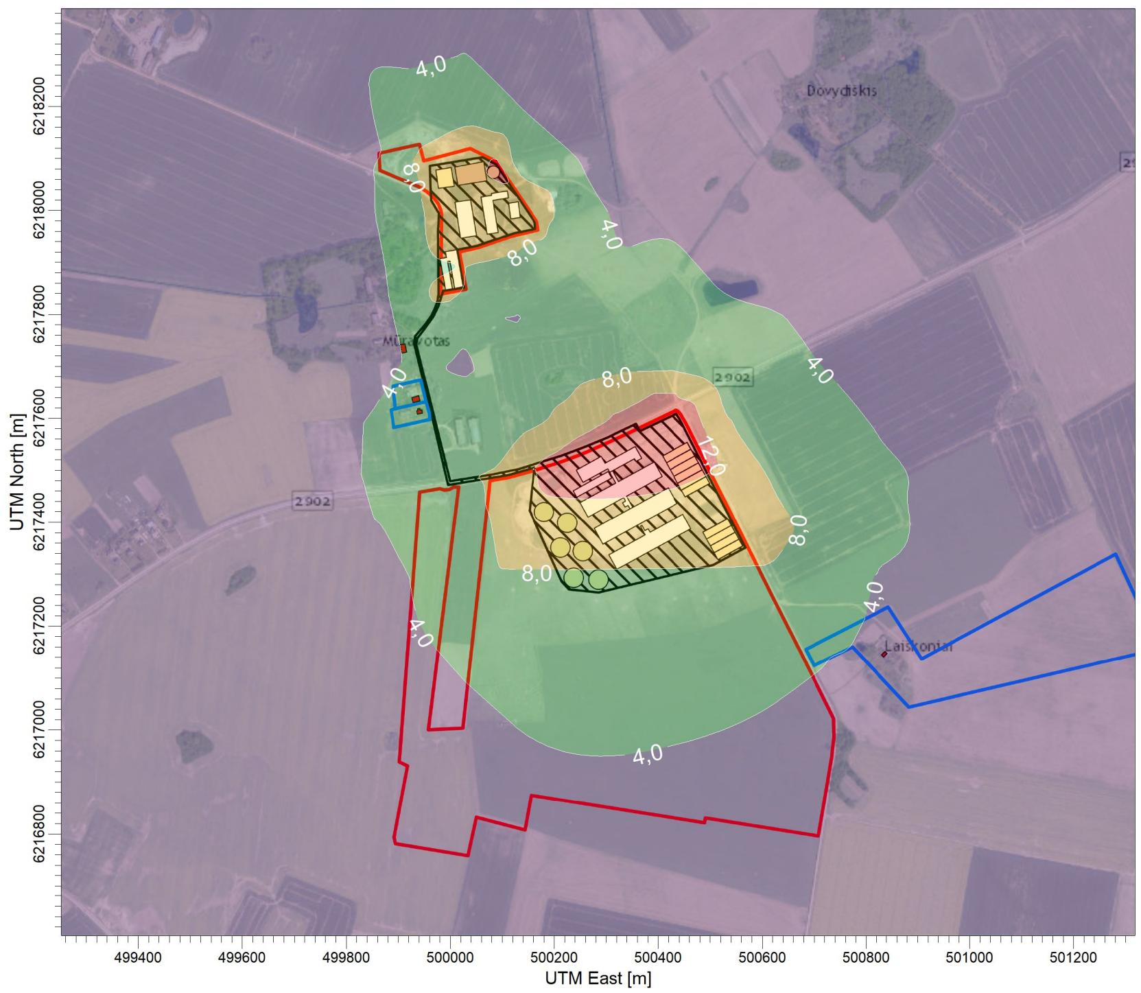
PLOT FILE OF HIGH 1ST HIGH 8-HR VALUES FOR SOURCE GROUP: PUV Max: 15,1 [ug/m 3 ] at (500435,32, 6217615,75)
