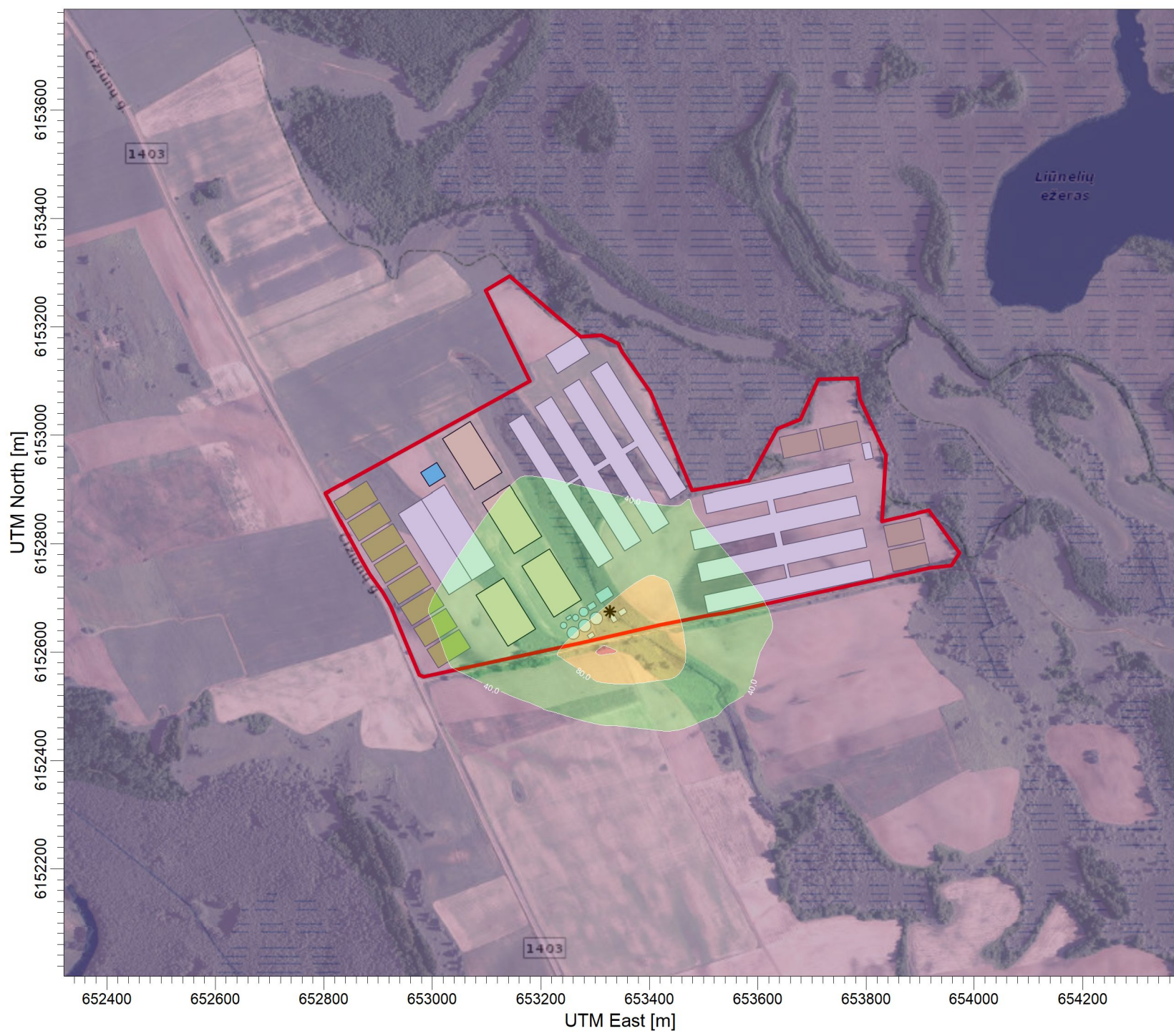
PLOT FILE OF 99.80TH PERCENTILE 1-HR VALUES FOR SOURCE GROUP: ALL Max: 123,9 [\mu\text{g}/\text{m}^3] at (653306,97, 6152599,97)
