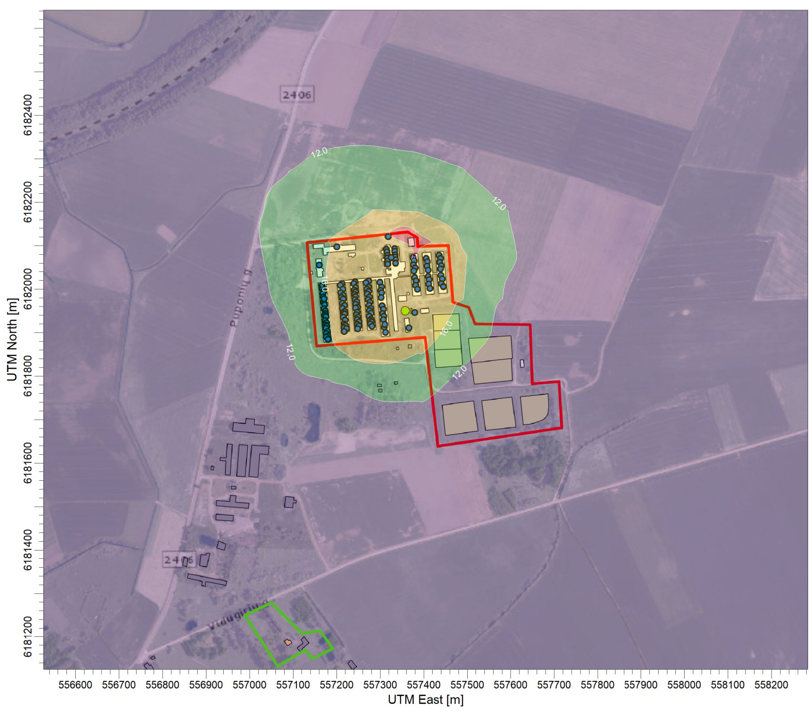
PLOT FILE OF ANNUAL VALUES AVERAGED ACROSS 5 YEARS FOR SOURCE GROUP: ALL Max: 21,5 [ug/m^3] at (557363,19, 6182130,47)
