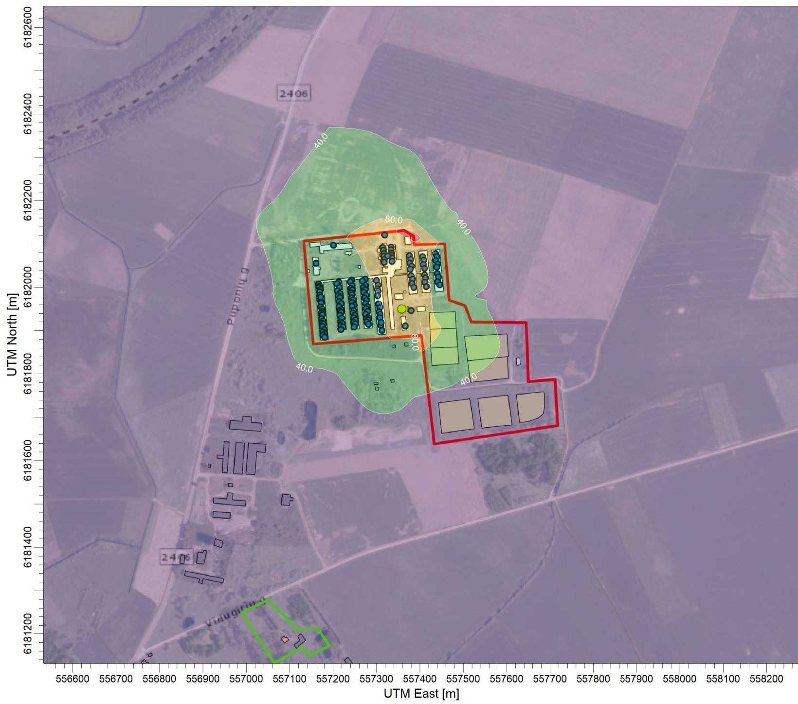
PLOT FILE OF 99.80TH PERCENTILE 1-HR VALUES FOR SOURCE GROUP: ALL Max: 122,5 [ug/m^3] at (557387,39, 6182117,12)
