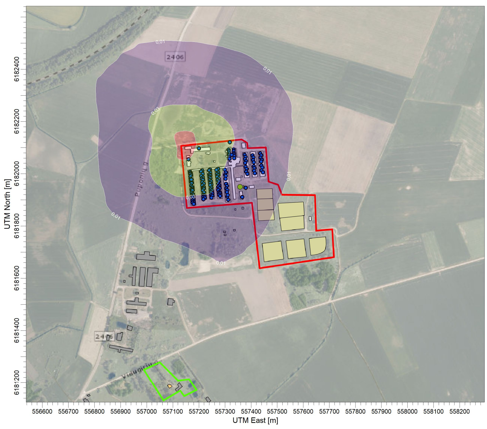
PLOT FILE OF 98.50TH PERCENTILE 1-HR VALUES FOR SOURCE GROUP: PUV Max: 0,06 [ \mu\text{g}/\text{m}^3 ] at (557132,87, 6182106,27)
