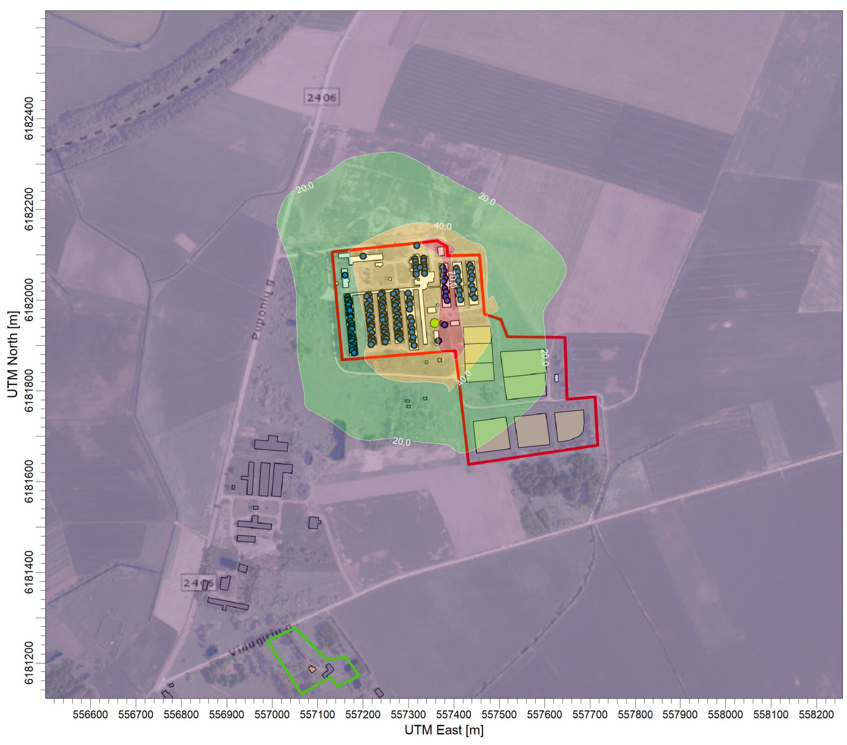
PLOT FILE OF 99.20TH PERCENTILE 24-HR VALUES FOR SOURCE GROUP: ALL Max: 82,2 [ \mu\text{g}/\text{m}^3 ] at (557403,25, 6181889,30)
