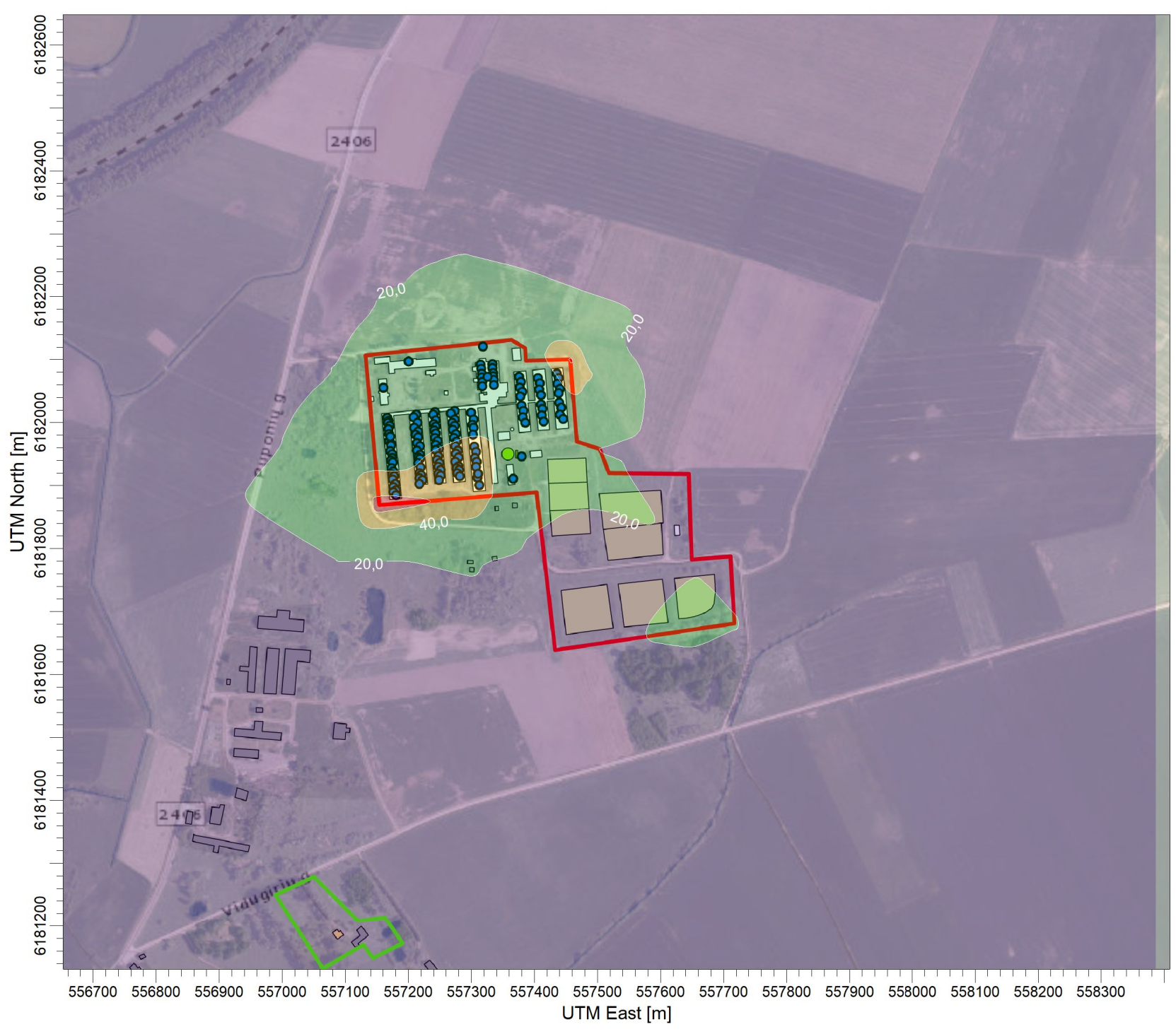
PLOT FILE OF HIGH 1ST HIGH 24-HR VALUES FOR SOURCE GROUP: ALL Max: 54,3 [ug/m^3] at (557154,57, 6181869,27)
