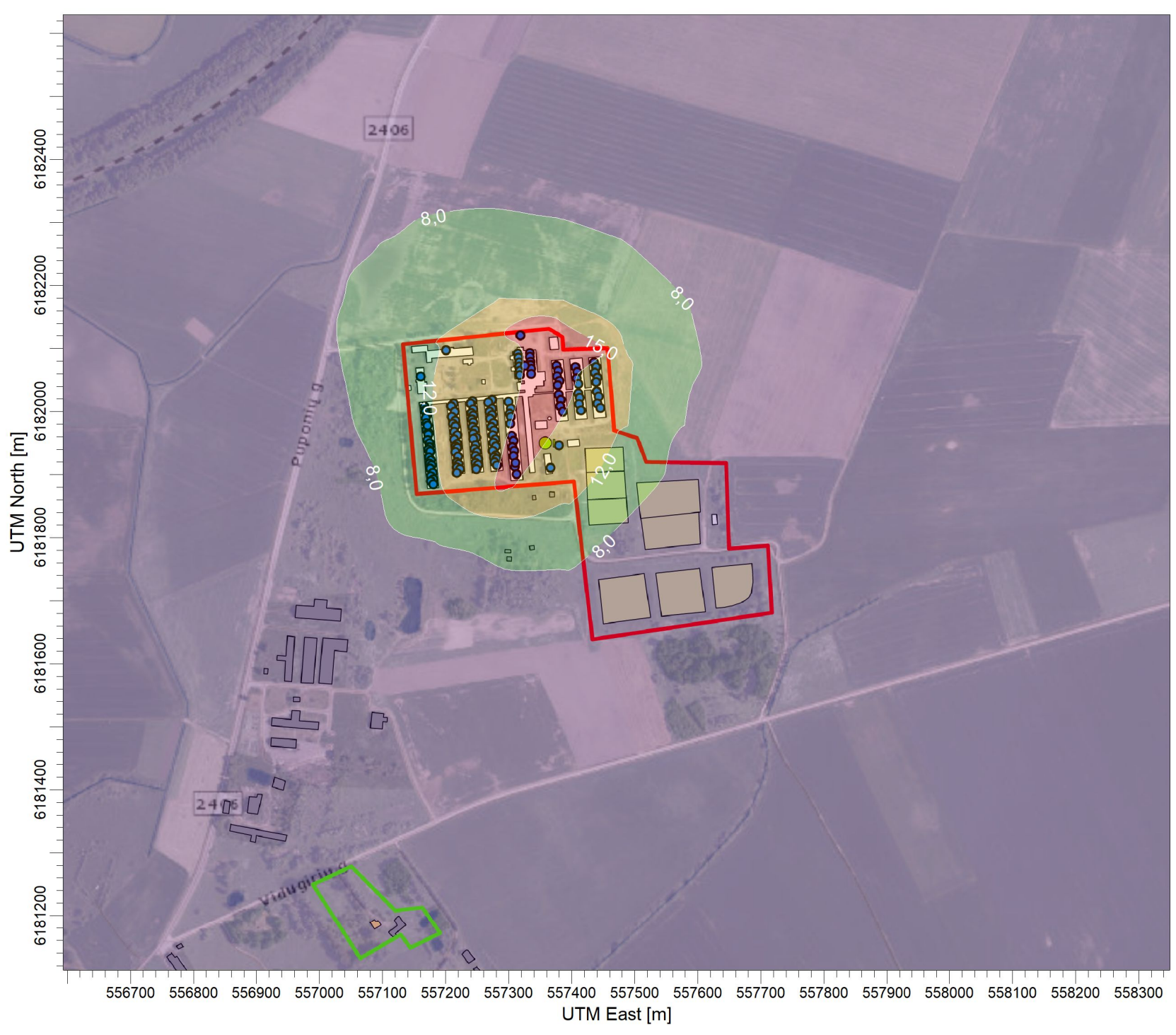
ug/m 3 PLOT FILE OF ANNUAL VALUES AVERAGED ACROSS 5 YEARS FOR SOURCE GROUP: ALL Max: 17,4 [ug/m 3 ] at (557363,19, 6182130,47)
