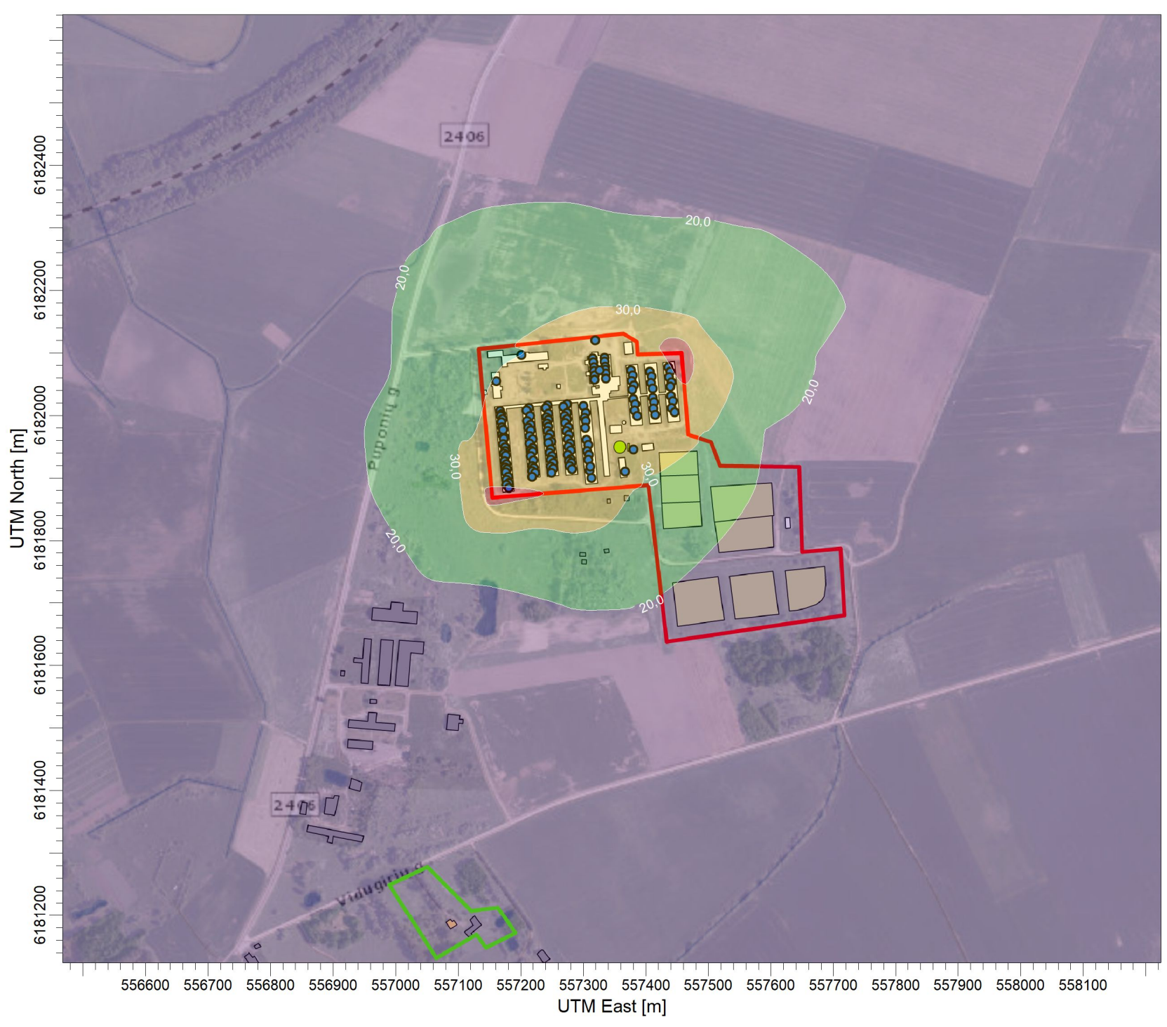
PLOT FILE OF 98.50TH PERCENTILE 1-HR VALUES FOR SOURCE GROUP: ALL Max: 45,5 [ug/m^3] at (557458,33, 6182099,60)
