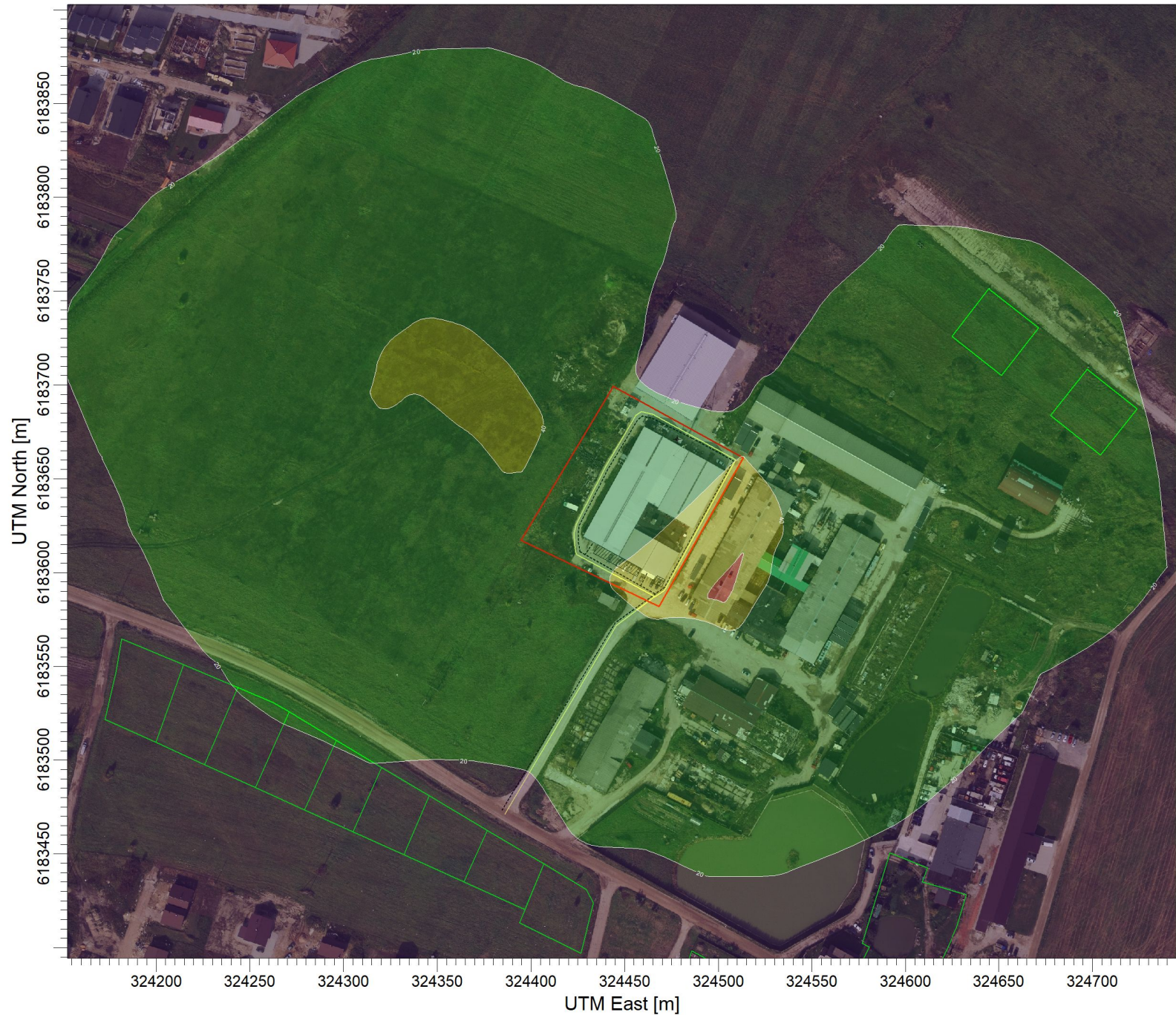
PLOT FILE OF 99.80TH PERCENTILE 1-HR VALUES FOR SOURCE GROUP: PŪV Max: 66,4 [ug/m^3] at (324501,49, 6183588,93)
