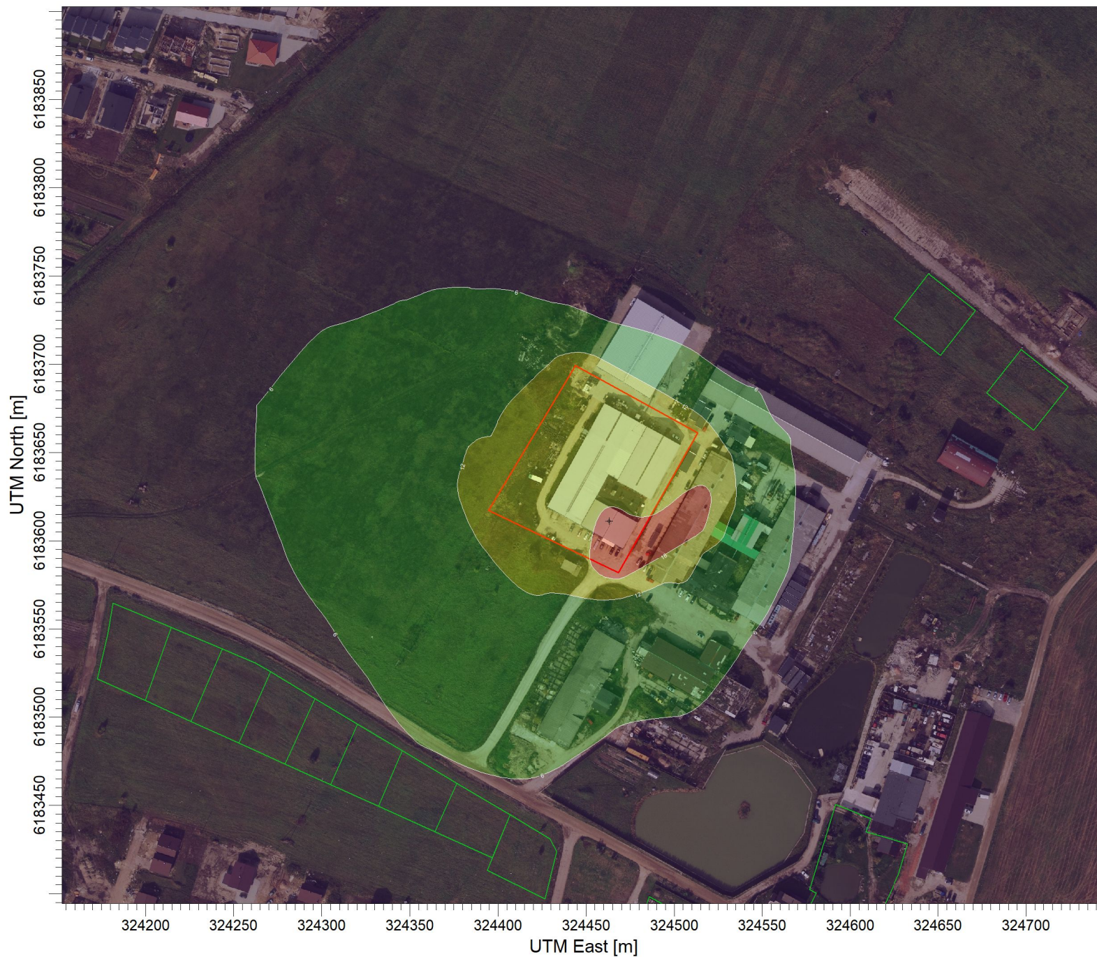
PLOT FILE OF 98.50TH PERCENTILE 1-HR VALUES FOR SOURCE GROUP: ALL Max: 20,6 [ \mu\text{g}/\text{m}^3 ] at (324512,67, 6183608,97)
