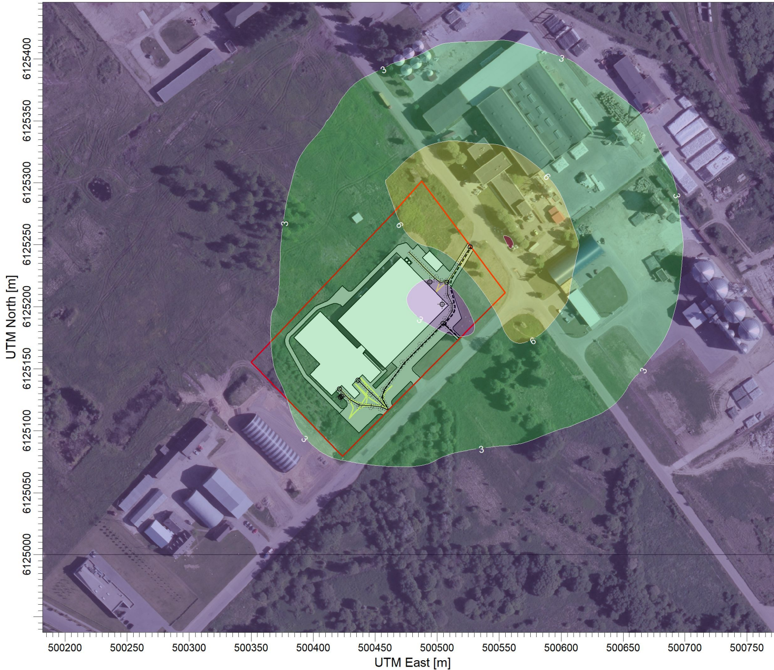
PLOT FILE OF ANNUAL VALUES AVERAGED ACROSS 5 YEARS FOR SOURCE GROUP: PŪV Max: 9,2 [ug/m^3] at (500558,88; 6125251,62)
