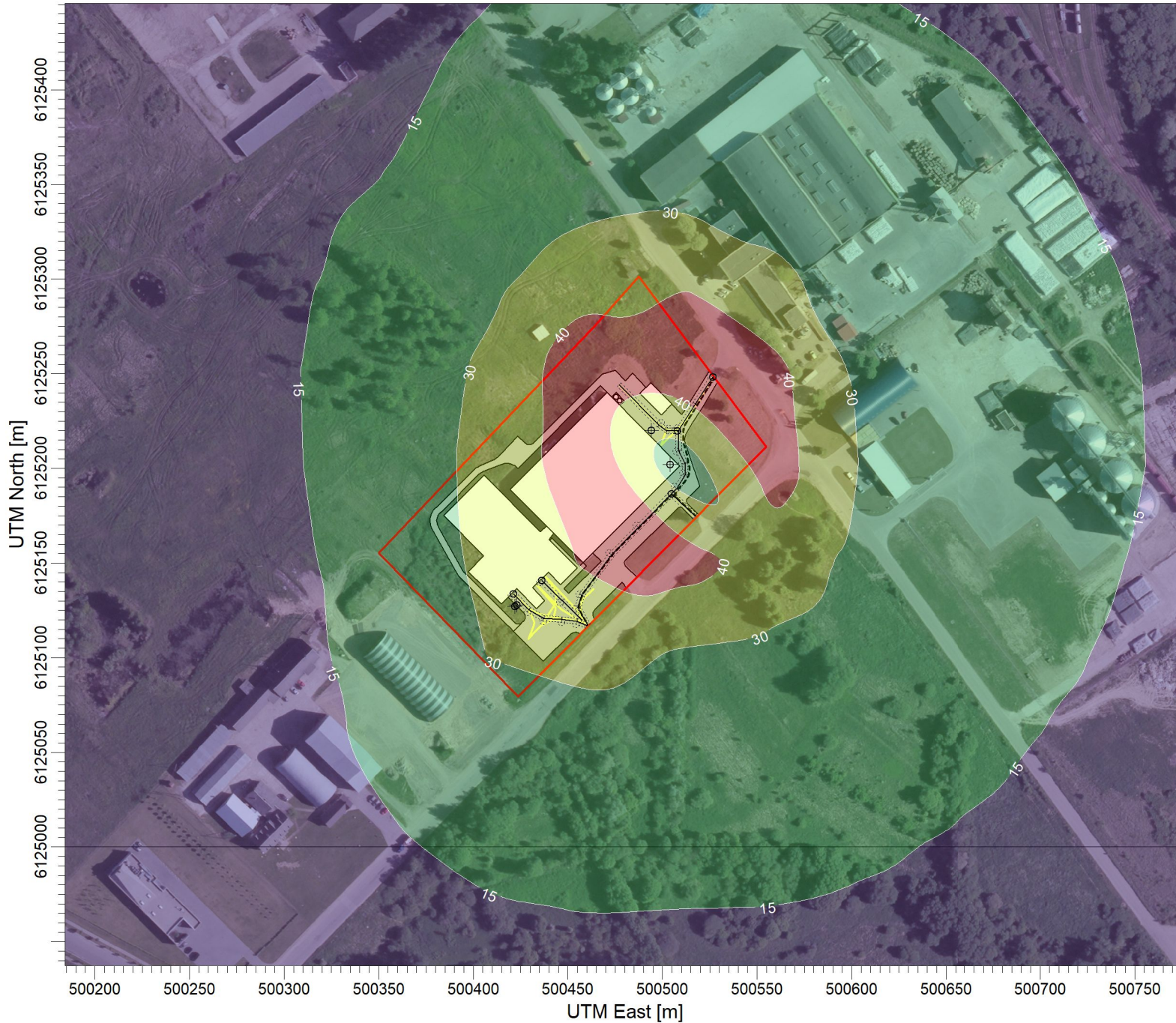
PLOT FILE OF 99.80TH PERCENTILE 1-HR VALUES FOR SOURCE GROUP: PŪV Max: 46,4 [ug/m^3] at (500458,88, 6125251,62)
