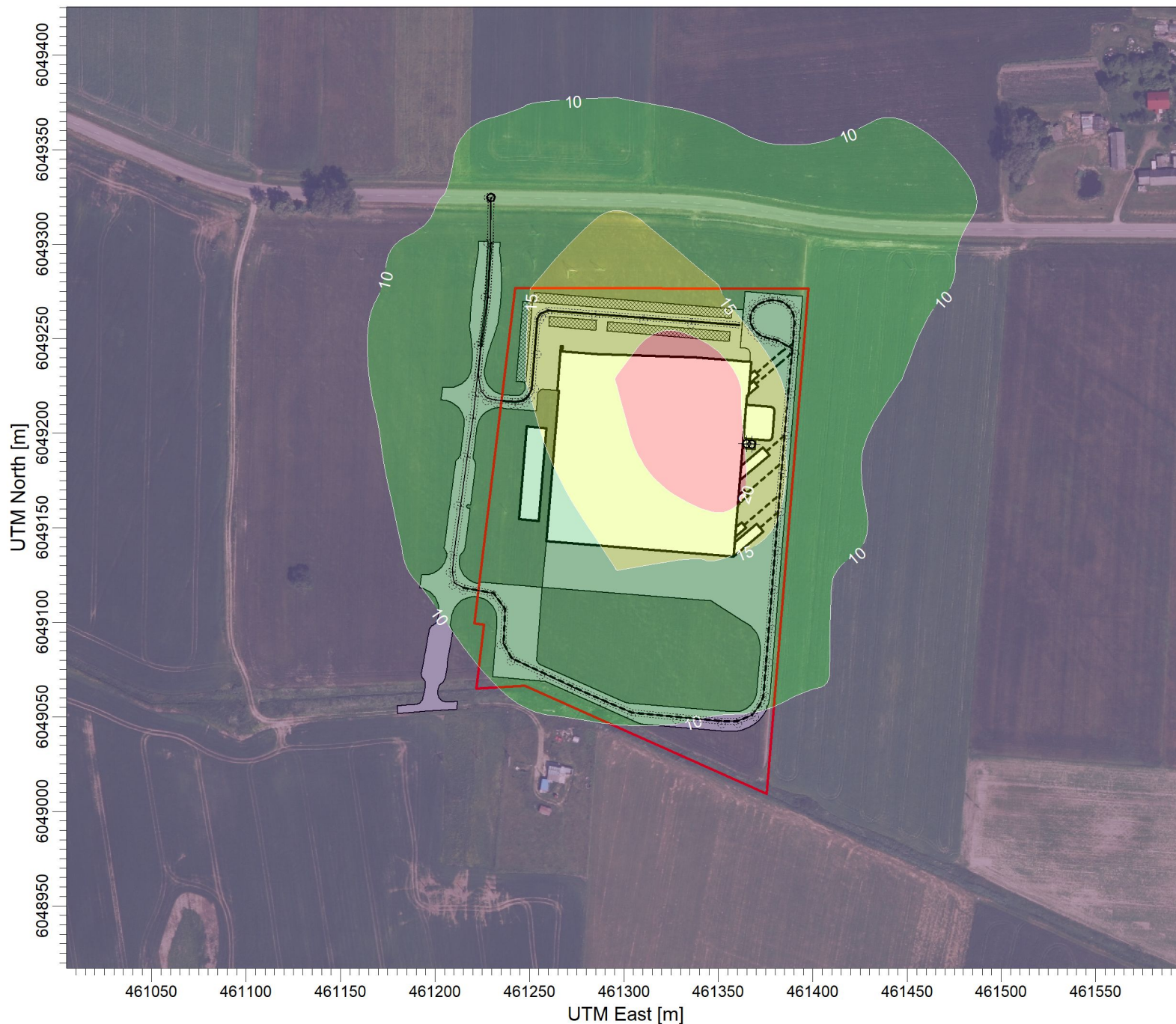
PLOT FILE OF ANNUAL VALUES AVERAGED ACROSS 5 YEARS FOR SOURCE GROUP: ALL Max: 24,6 [ug/m^3] at (461346,39, 6049178,22)
