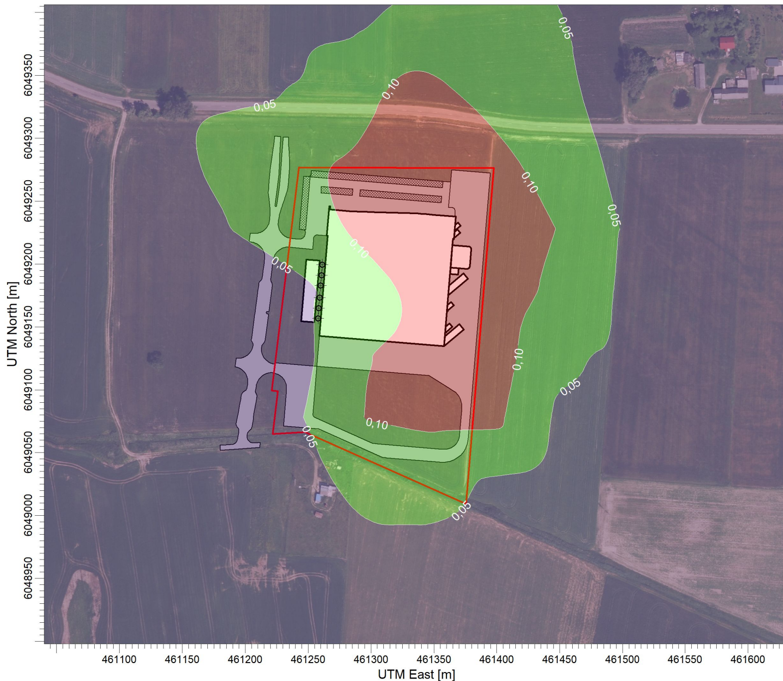
PLOT FILE OF 98.50TH PERCENTILE 1-HR VALUES FOR SOURCE GROUP: PŪV Max: 0,16 [ \mu\text{g}/\text{m}^3 ] at (461346,39, 6049278,22)
