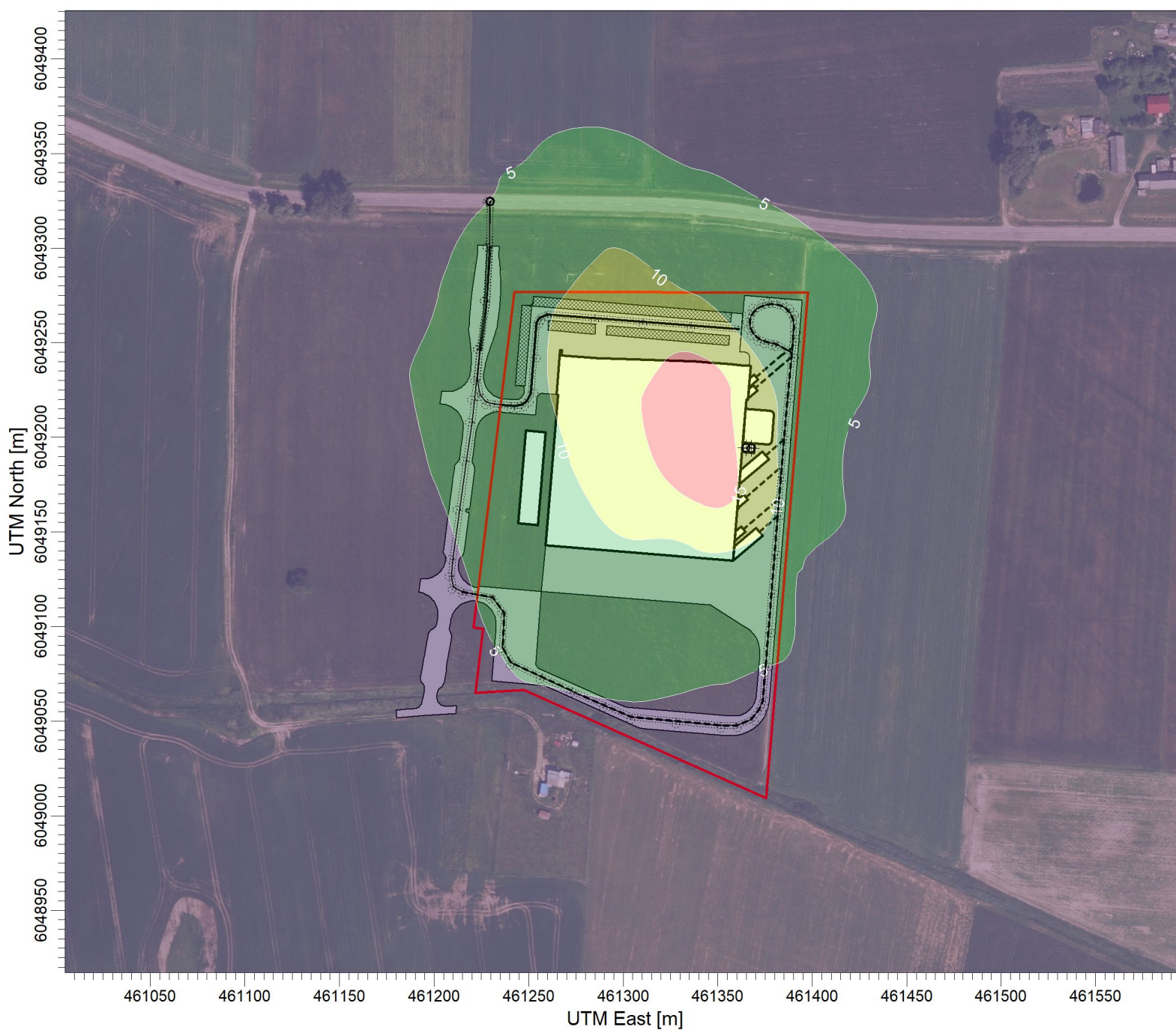
PLOT FILE OF ANNUAL VALUES AVERAGED ACROSS 5 YEARS FOR SOURCE GROUP: PŪV Max: 18,5 [ug/m 3 ] at (461346,39, 6049178,22)
