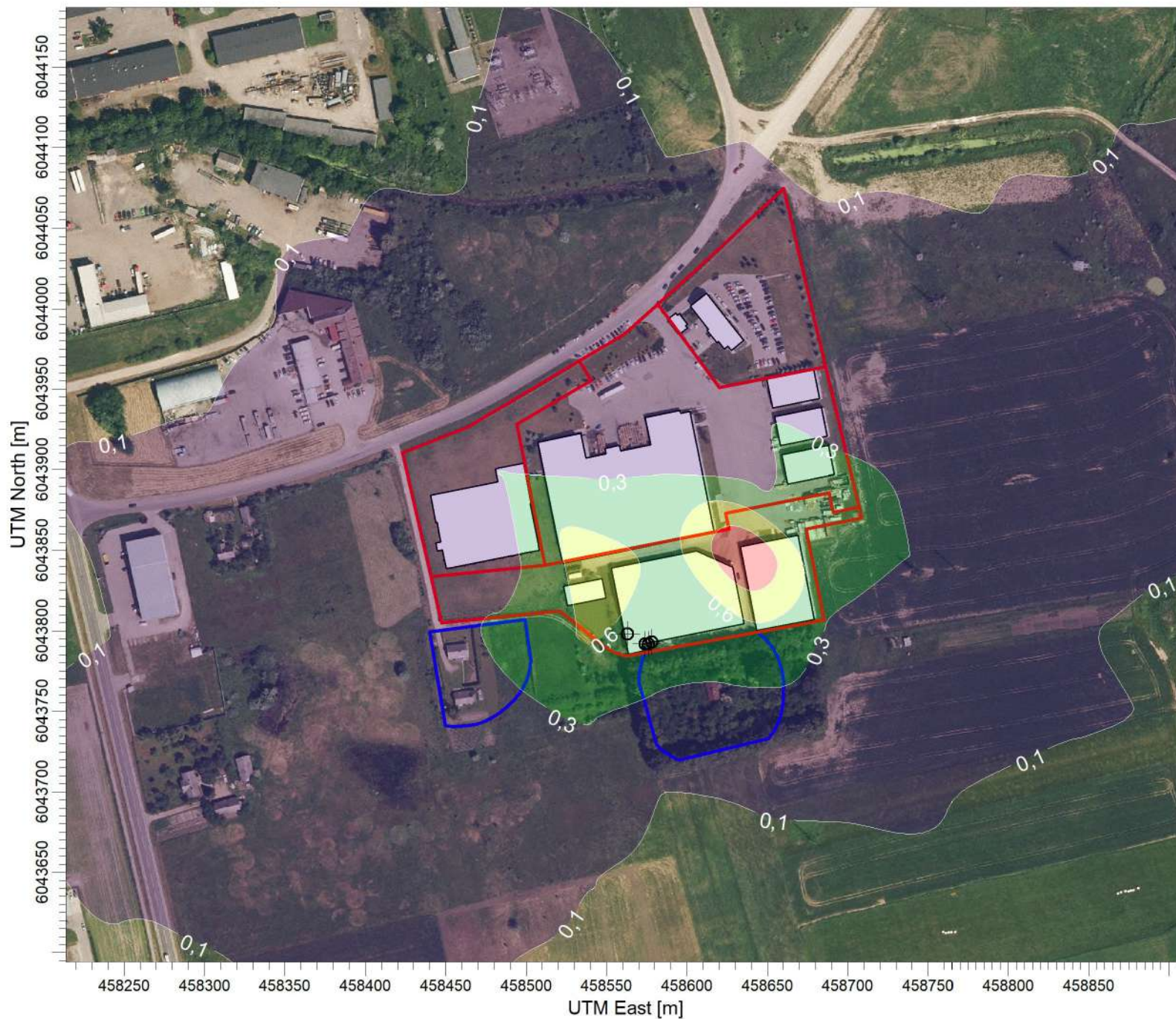
PLOT FILE OF HIGH 1ST HIGH 24-HR VALUES FOR SOURCE GROUP: NH3 Max: 1,2 [ug/m 3 ] at (458637,13, 6043847,42)
