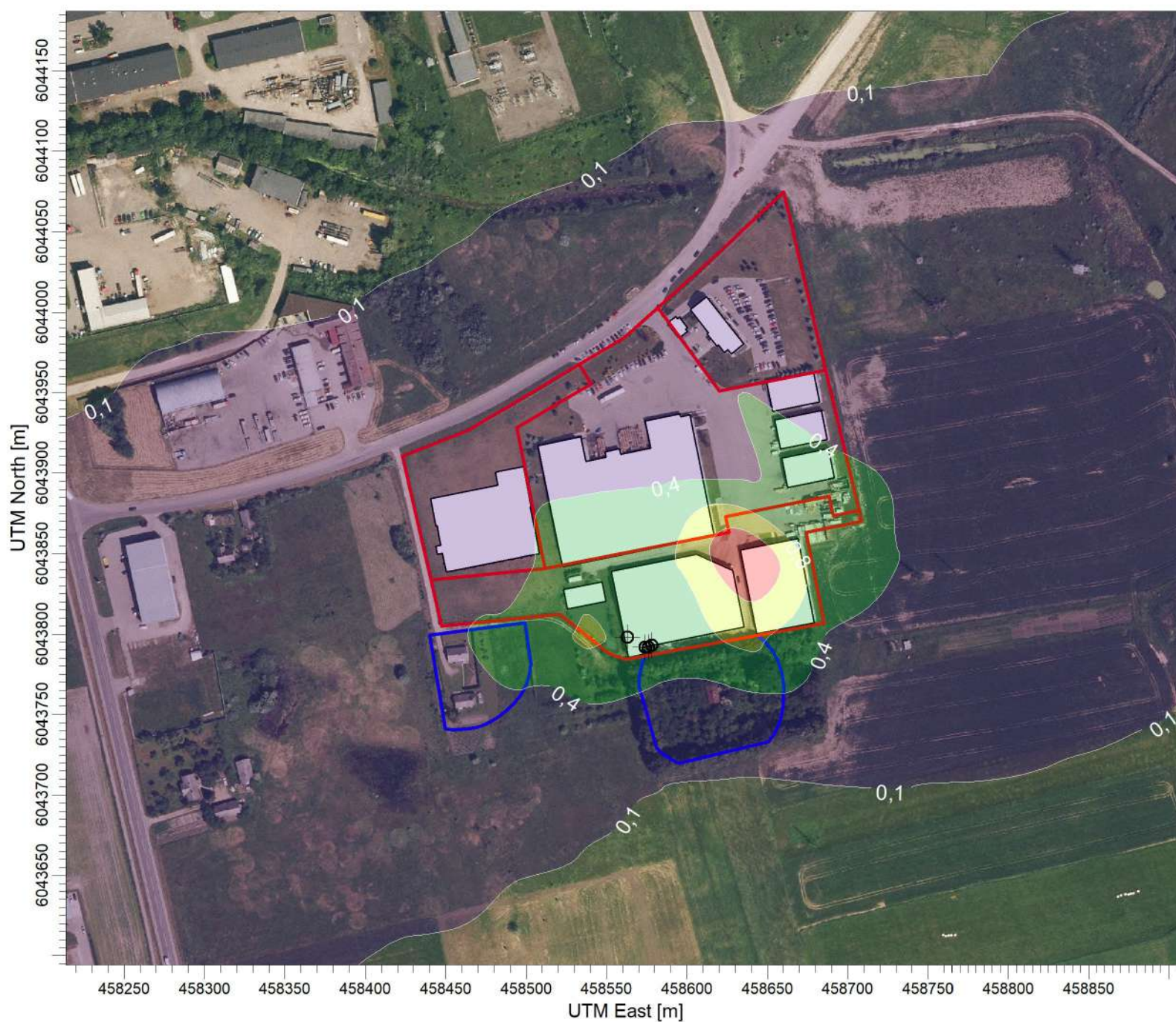
PLOT FILE OF 98.50TH PERCENTILE 1-HR VALUES FOR SOURCE GROUP: NH3 Max: 1,7 [ug/m^3] at (458637,13, 6043847,42)
