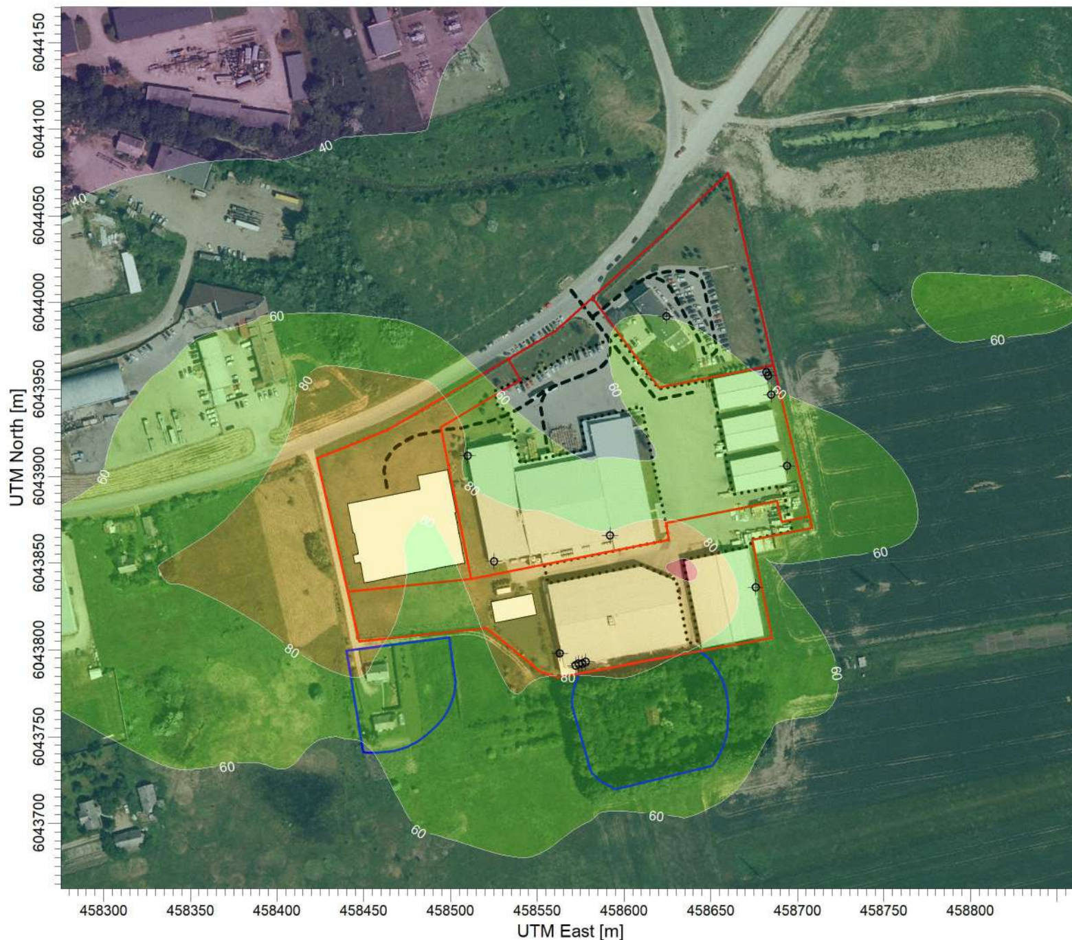
PLOT FILE OF 99.80TH PERCENTILE 1-HR VALUES FOR SOURCE GROUP: ALL Max: 104,6 [ug/m^3] at (458637,13, 6043847,42)
