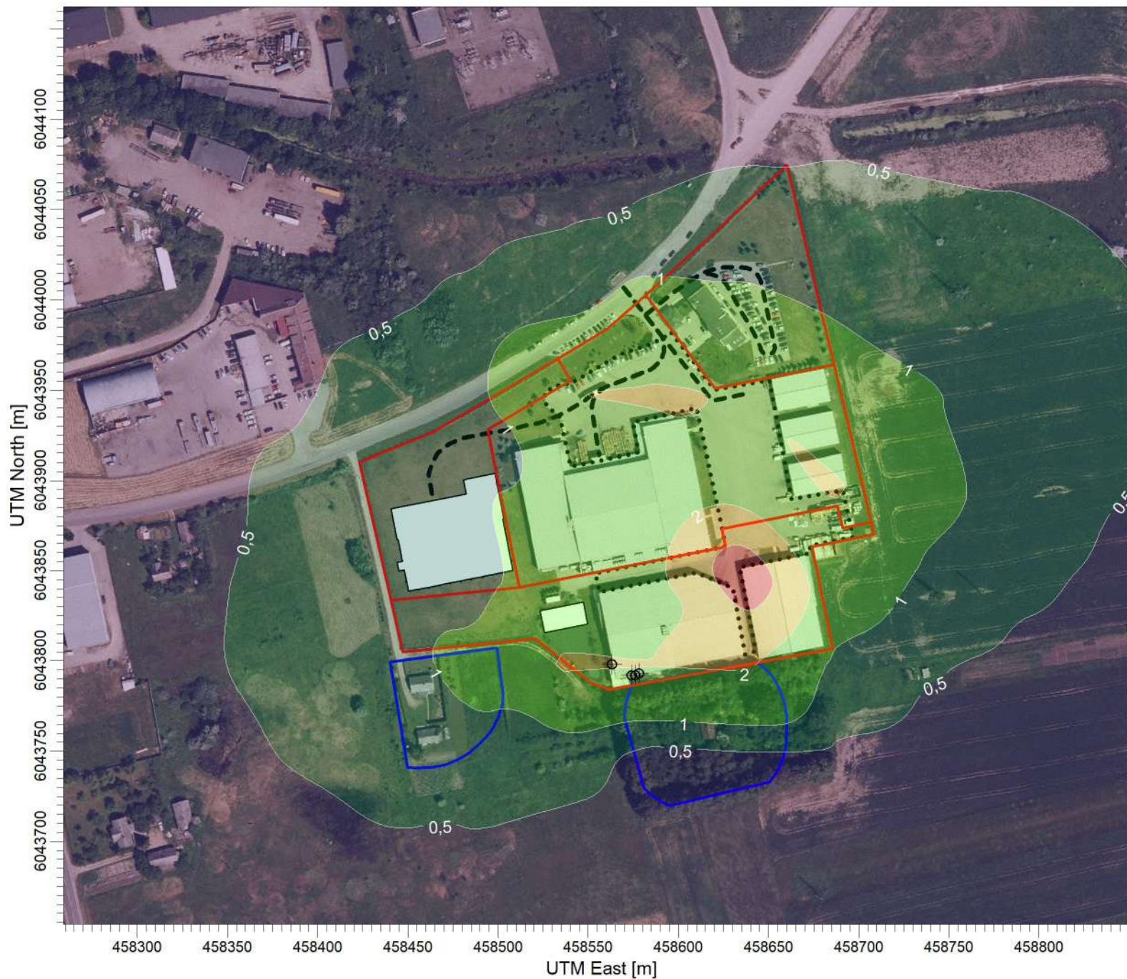
PLOT FILE OF 90.40TH PERCENTILE 24-HR VALUES FOR SOURCE GROUP: KD10 Max: 3,7 [ug/m^3] at (458637,13, 6043847,42)
